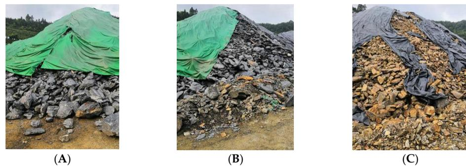
**Figure 1.** Classification of aggregate in engineering site. (A) slightly weathered material; (B) weakly weathered material; (C) strongly weathered material.
