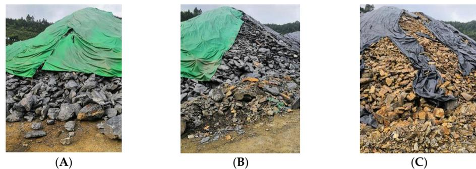
**Figure 1.** Classification of aggregate in engineering site. (A) slightly weathered material; (B) weakly weathered material; (C) strongly weathered material.
