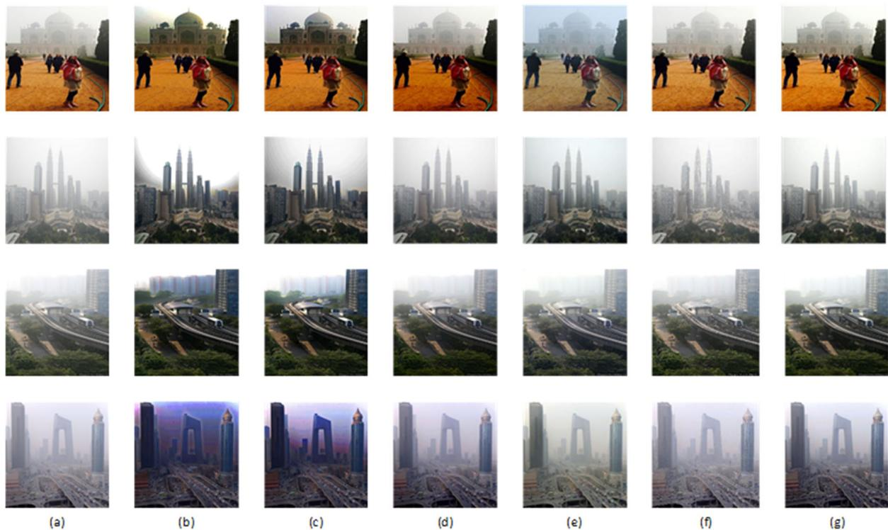
**Figure 7.** The experimental results of the real outdoor hazy images. (a) Hazy image; (b) method in [5]; (c) method in [6]; (d) method in [11]; (e) method in [12]; (f) method in [15]; (g) proposed method.
