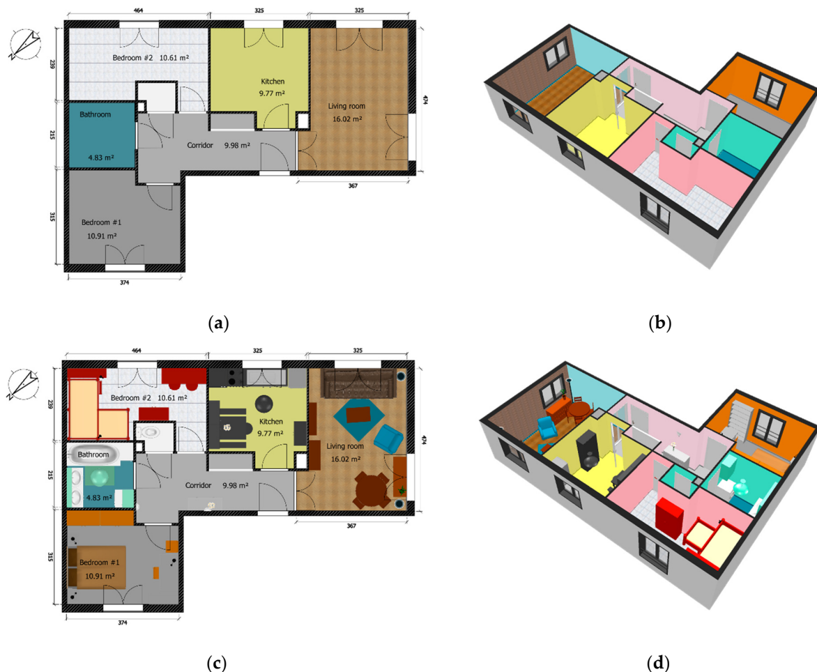
Figure 2. Design of an apartment using the software Sweet Home 3D: 2D plan and 3D representation of the unfurnished apartment are depicted in (a,b), respectively; (c,d) are the equivalents of furnished designs.
