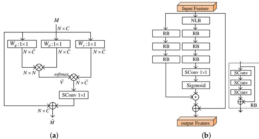
**Figure 2.** (a) non-local block.  $\oplus$  is the add operation and  $\otimes$  is the matrix multiplication. (b) non-local attention module.  $\odot$  means element-wise product.
