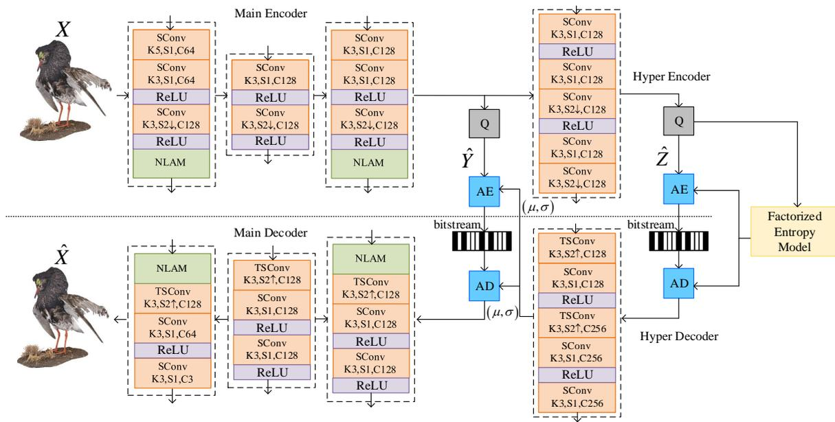
**Figure 1.** The proposed autoencoder network with non-local attention mechanism module. “SConv K3, S2↓, C128” indicates a downsampling sparse convolution layer with a kernel of size 3 × 3 × 3, stride of 2, and 128 output channels. “TSConv” with “S2↑” stands for upsampling transposed sparse convolution layers with stride of 2. “ReLU” represents the Rectified Linear Unit. NLAM refers to non-local attention modules. “Q” is for quantization. “AE” and “AD” are arithmetic encoding and decoding.
