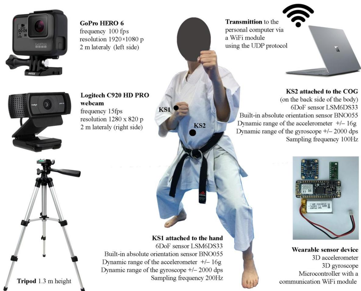
**Figure 1.** The experimental set-up included two cameras and a laptop wirelessly connected to two sensors attached to the athlete.
