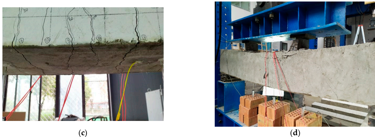
Figure 5. Beam L-1-30 experimental phenomena. (a) Development of cracks on the front of beam L-1-30; (b) the concrete on the upper part of the beam L-1-30 is crushed; (c) a through crack at the bottom of beam L-1-30; (d) development of cracks on the back of beam L-1-30.
