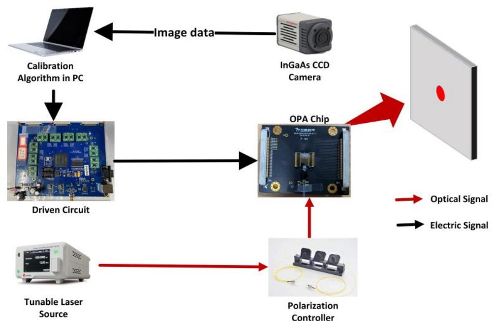
**Figure 1.** The phase calibration system of an OPA.
