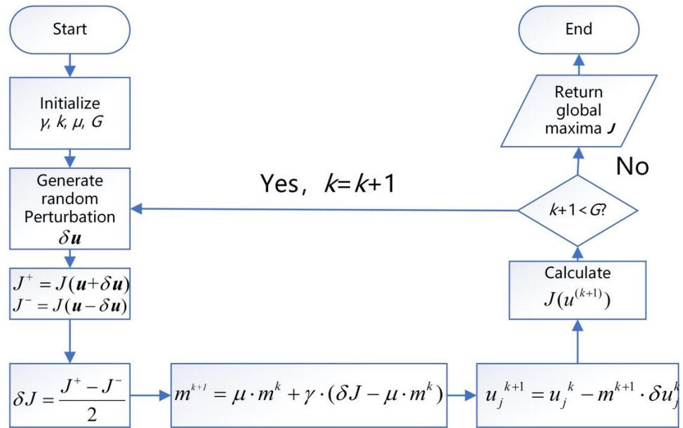
Figure 2. Flow chart of NSPGD algorithm.
