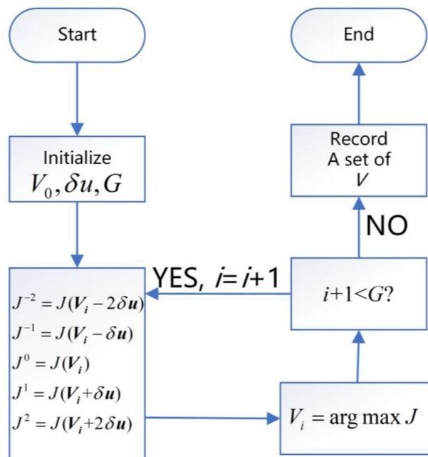
Figure 3. Flow chart of HC algorithm.
