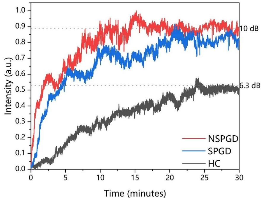
**Figure 4.** Convergence time of NSPGD, SPGD, and HC on 512-channel OPA.
