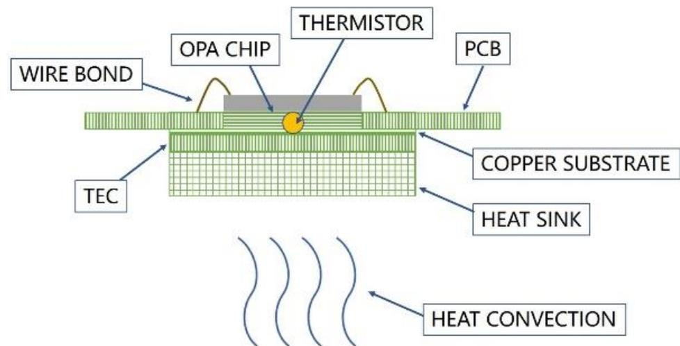
**Figure 5.** Schematic of 512-channel OPA with temperature-controlled packaging.
