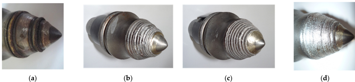
Figure 5. Variants of alloyed powder and laser metal deposition on the frustoconical section of the tooth; (a) two cord metal deposition; (b) metal deposition with a one-third overlap; (c) metal deposition with a two-third overlap; (d) optimized metal deposition.
