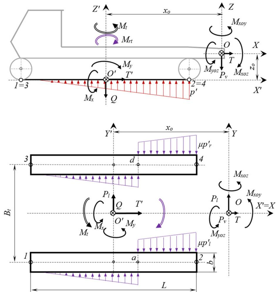
Figure 4. Scheme of determining the moment of resistance of the tractor turn.
