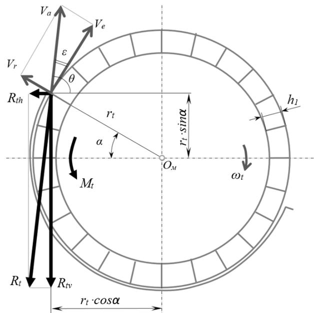
Figure 7. Calculation scheme for determining the loading of the soil thrower.
