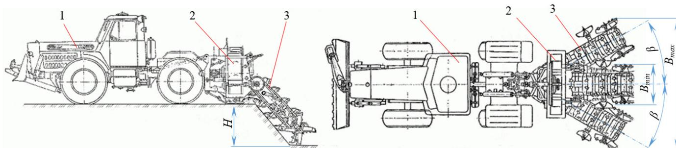
**Figure 1.** Machinery for digging trenches of variable width: 1—basic tractor; 2—rotary soil evacuator; 3—chain soil development actuator;  $H$ —digging depth;  $B_{min}$ —the minimum excavation width;  $B_{max}$ —the maximum excavation width;  $\beta$ —the angle of rotation of the actuator.
