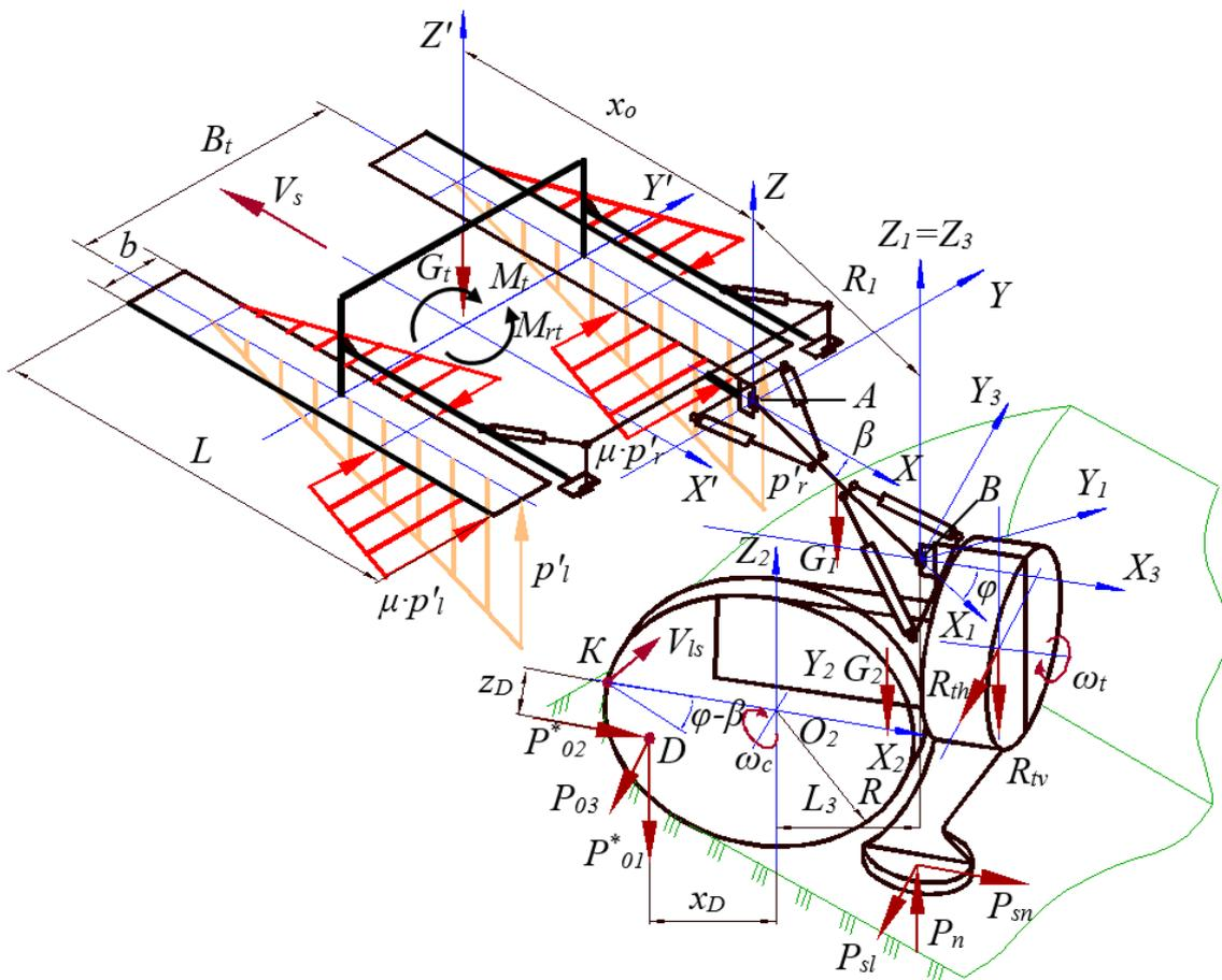
**Figure 3.** Calculation scheme of power loading of the machinery.
