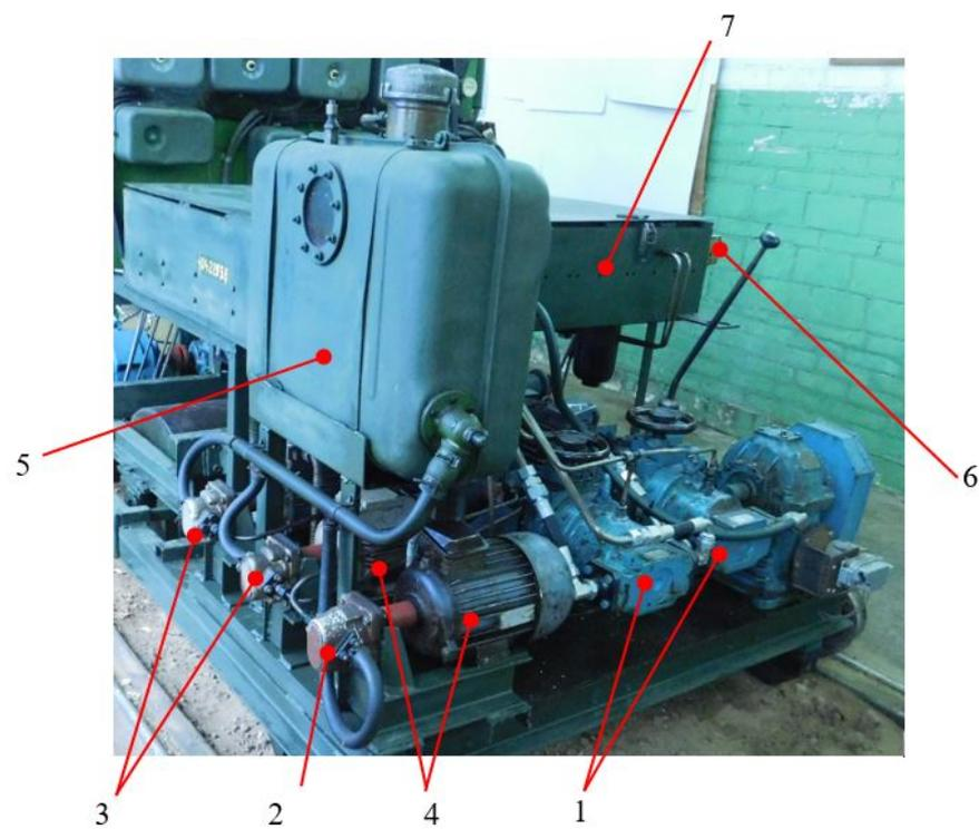
**Figure 10.** A pump station (1—adjustable pump NAR-40/200; 2—gear pump NCH-6; 3—gear pump NCH-10; 4—electric motor; 5—tank; 6—flow regulator; 7—station hydraulic panel).
