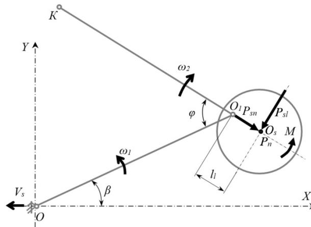
Figure 8. Calculation scheme for determining the loading of the sweeping shoe.
