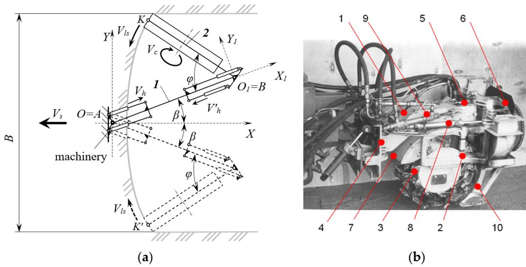
**Figure 2.** Universal continuous earthmoving machinery (UEM) rotor operating equipment: (a) layout scheme; (b) physical model of equipment (1—intermediate frame; 2—rotor frame; 3—rotor; 4—vertical hinge aft of the machinery; 5—hinge connecting the rotor frame and the intermediate frame; 6—thrower; 7—rotor housing; 8—hydraulic cylinders of rotor frame rotation; 9—hydraulic cylinders of intermediate frame rotation; 10—sweeping support shoe).
