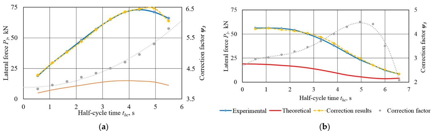
**Figure 12.** Change of lateral force on the operating equipment of the universal earthmoving machinery during the half-cycle: (a) without the intermediate frame rotation; (b) with the intermediate frame rotation ( $C = 15$ ,  $B = 4.5$  m,  $V_{ls} = 0.7$  m/s,  $V_c = 6$  m/s,  $V_s = 104$  m/h).
