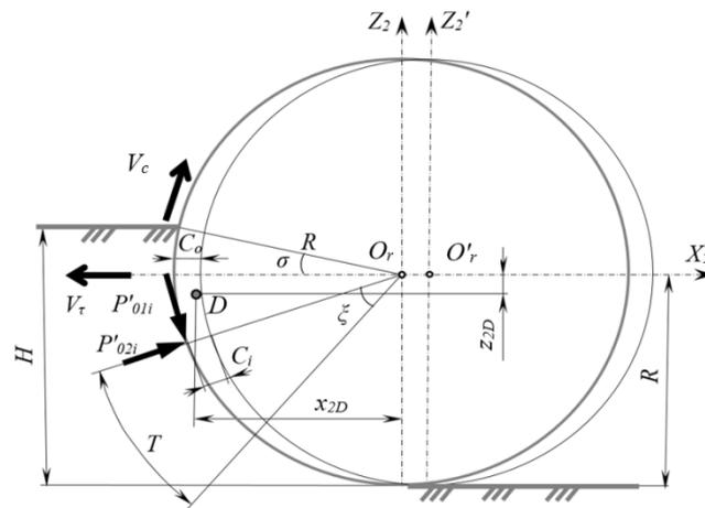
Figure 5. Calculation scheme for determining the resistance to frontal cutting of the soil with the rotor buckets.
