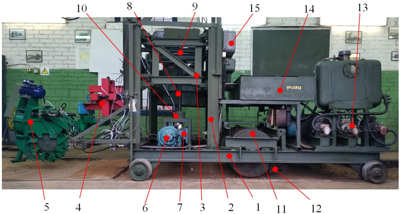
**Figure 9.** General view of the test bench with a model of the actuator (1—main frame; 2—frame; 3—carriage; 4—strain gauge; 5—actuator; 6—reversible motor; 7—worm gearbox; 8—lead screw; 9—upper ball bearing; 10—lower ball bearing; 11—roller; 12—profiling device; 13—pump station; 14—station hydraulic panel; 15—starter panel).
