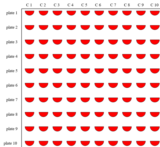
Figure 4. Schematic diagram of the PCHE inner layer number and flow channel number.
