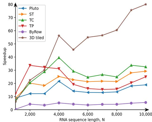
**Figure 4.** Speedup for Intel Xeon E5-2699 v3 and 36 threads.
