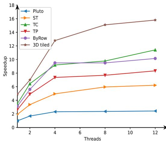
Figure 3. Speedup for Intel i7-8700 and RNA sequence length,  $N = 10,000$ .
