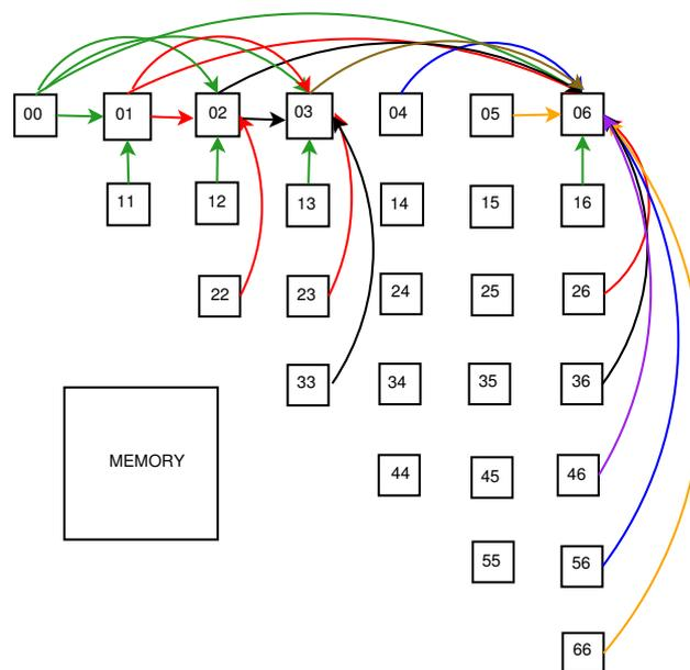
Figure 1. Calculation model to update cells.
