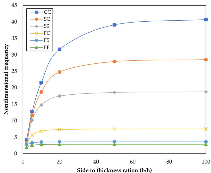
**Figure 7.** Effect on the non-dimensional frequency of the square orthotropic plate for the Levy-type boundary condition with a side-thickness ratio ( $b/h$ ) and the given value of Young's modulus ratio ( $\frac{E_1}{E_2} = 40$ ).
