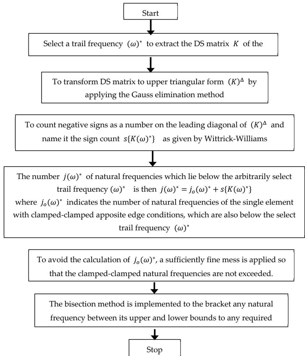
Figure 5. Flow chart for implementing the W-W algorithm.
