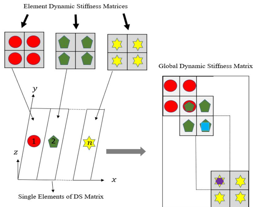
**Figure 4.** Assembly procedure of dynamic stiffness matrices.
