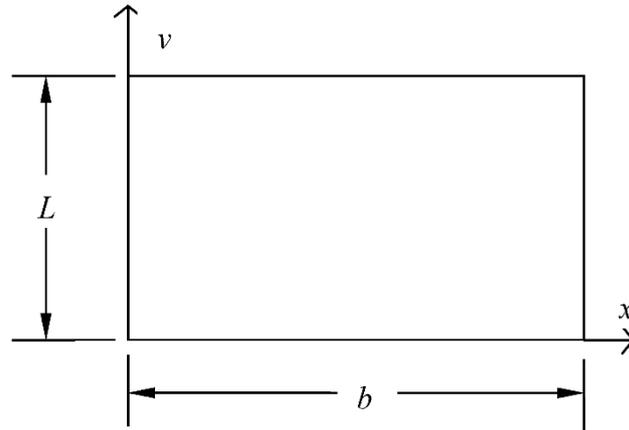
Figure 1. Levy-type solution boundary conditions with coordinate system convention.
