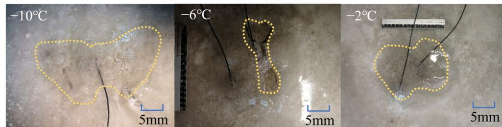
**Figure 11.** The actual deicing effect of each specimen at different initial temperatures.
