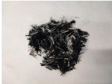
**Figure 1.** Basic morphology of carbon fiber after cutting.
