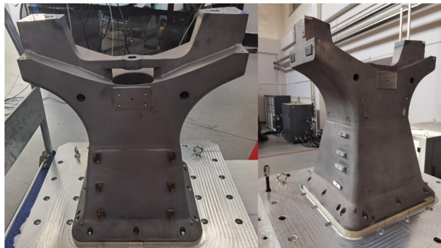
**Figure 8.** The printed model of the vertical bracket manufactured by SLM.
