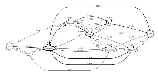
**Figure 5.** State diagram of the attacker's behaviour on Asgard.
