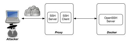
Figure 2. The architecture of proxy-based honeypots.
