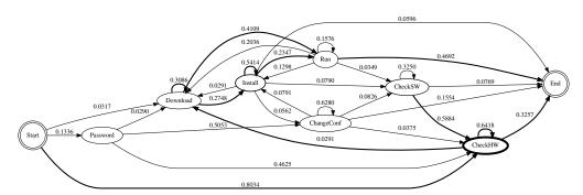
**Figure 7.** State diagram of the attacker's behaviour on Cowrie.
