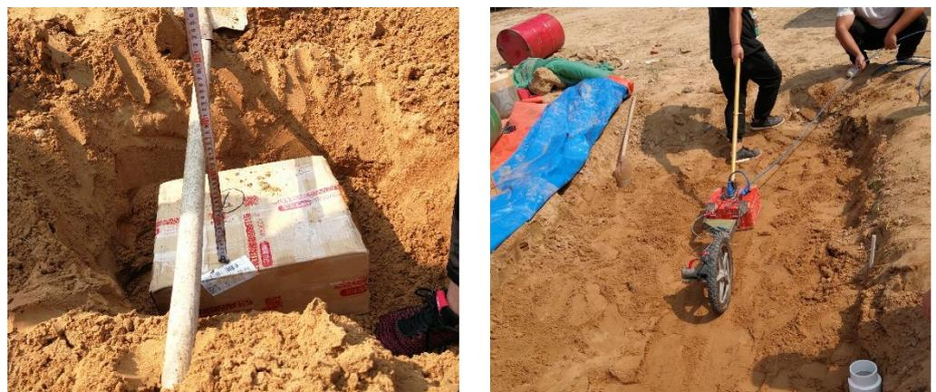
Figure 18. Road radar rectangular cavity experimental diagram.
