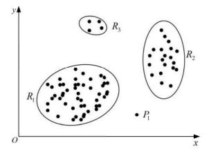
Figure 1. An example of two-dimensional data anomaly detection.
