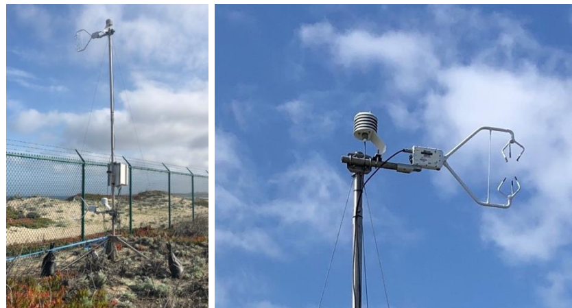
Figure 1. Sensor platform (left) and close-up of two of the sensors (right). The upper sensor is a HygroVUE5 hygrometer, and the one on the right is a CSAT3 sonic anemometer.
