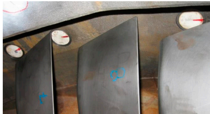
Figure 2. Sensors mounted in the casing of steam turbine LP last stage [27].
