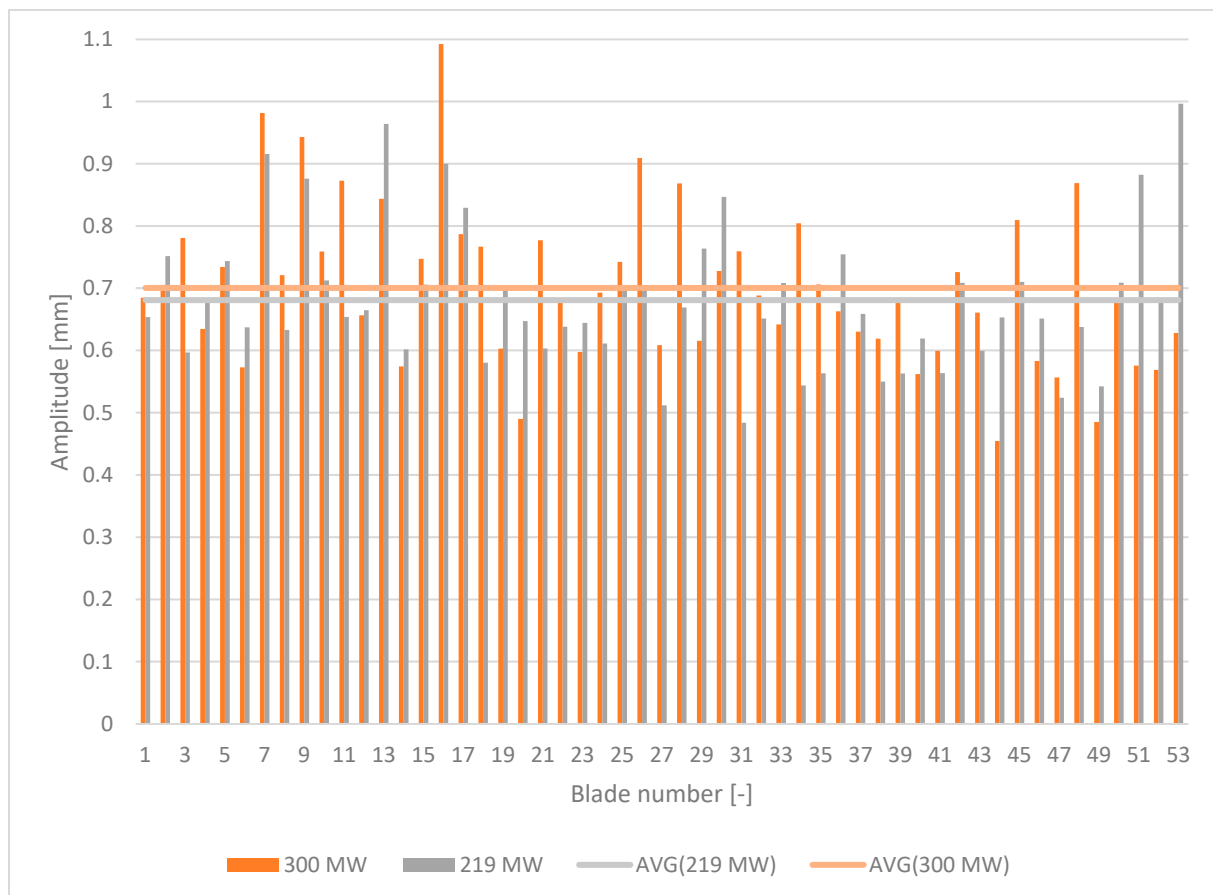
Figure 20. Blade amplitudes of 53 blades at various powers (measurements 2 and 3).
