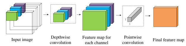
Figure 4. Depthwise separable convolution.
