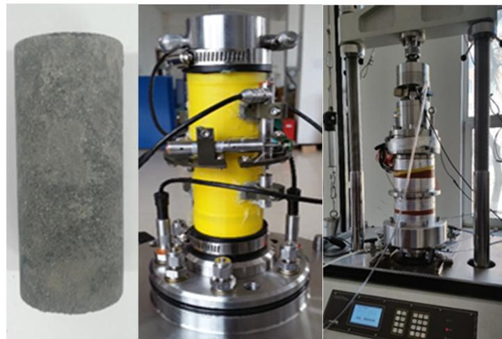
Figure 6. Test specimens and experimental setup.
