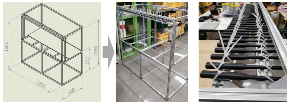
**Figure 4.** Originally designed and assembled sensor mount.
