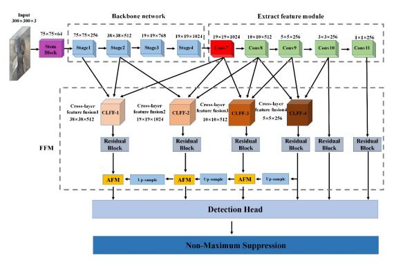
Figure 8. Tramp materials in raw coal single-shot detector (TMRC-SSD) architecture overview.
