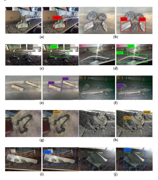
Figure 10. Visualization results. In the sub-figure (a-j), the left is the original picture, and the right is the visualization result of the proposed network. The sub-figures (a,b) show the detection of gangue; the sub-figures (c,d) show the detection of bolt; the sub-figures (e,f) show the detection of stick; the sub-figures (g,h) show the detection of iron sheet.
