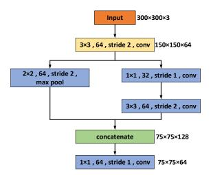
Figure 2. Schematic diagram of stem block.
