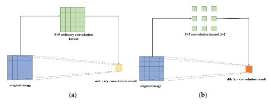
**Figure 3.** Dilation convolution operation. (a) The process of  $5 \times 5$  general convolution Convolve. (b) The process of  $3 \times 3$  dilated convolution (d = 2).
