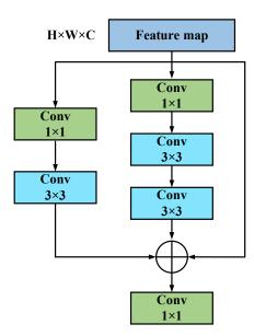
Figure 7. Schematic diagram of attention residual block.
