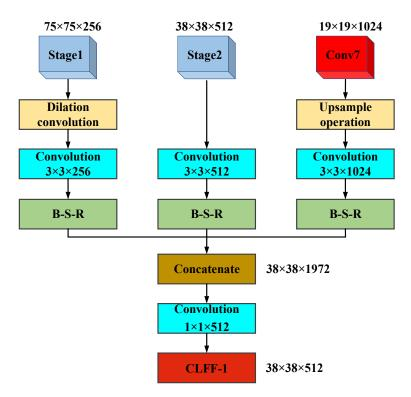
Figure 5. Schematic diagram of Cross-layer feature fusion-1(CLFF-1).
