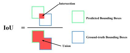
Figure 9. Schematic diagram of IoU.
