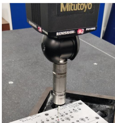
Figure 1. Hole geometry measurement setup using CMM.
