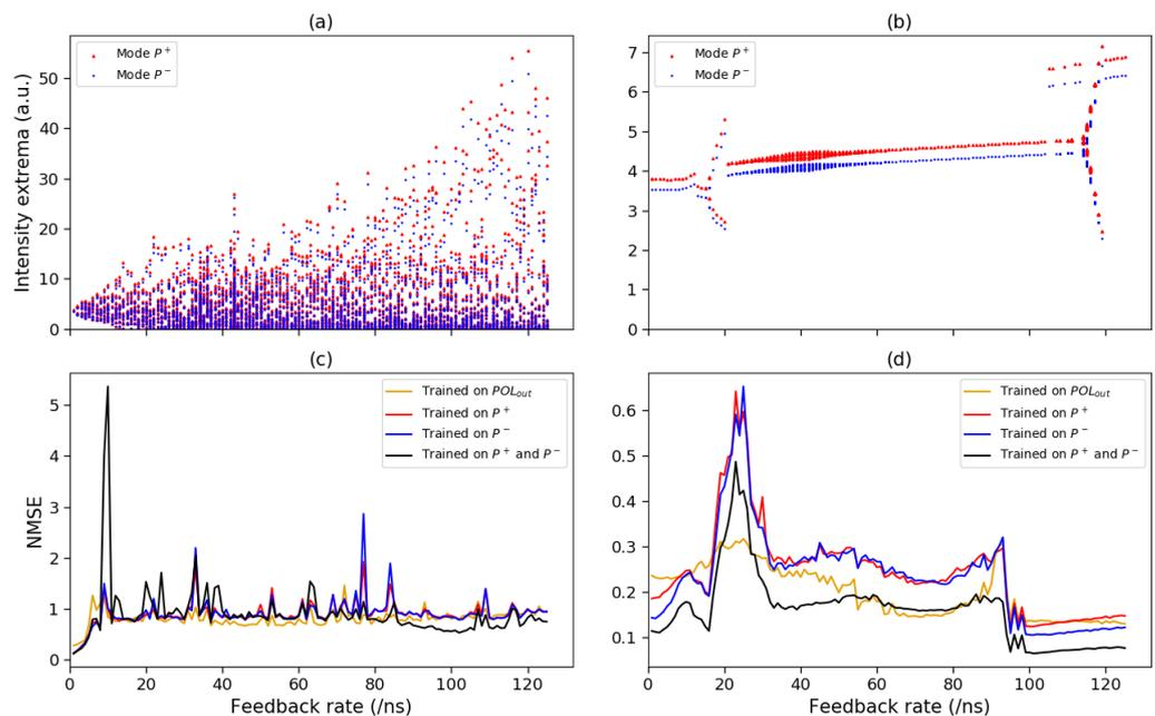
**Figure 3.** Orbit diagram of the modal output power as the feedback rate  $\eta$  is varied for (a)  $\tau_D = 150$  ps and (b)  $\tau_D = 15$  ps. The NMSE for the Santa Fe timeseries prediction task as the feedback is varied for (c)  $\tau_D = 150$  ps and (d)  $\tau_D = 15$  ps.
