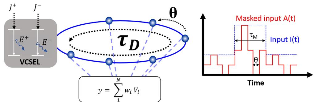
**Figure 1.** (left) Schematic overview of our setup, consisting of a spin-VCSEL connected to a feedback line with delay  $\tau_D$ . The spin-up and spin-down populations are pumped separately by  $J^+$  and  $J^-$ , respectively. (right) A simplified plot showing the input data  $I(t)$  in blue, the masked input data  $A(t)$  in red and the timescales of  $\tau_M$  and  $\theta$ .
