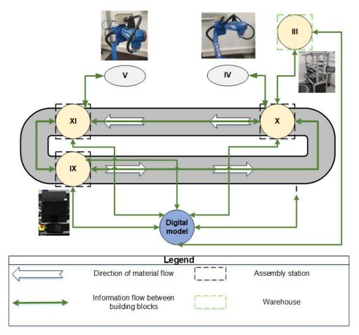
Figure 15. Connections between the digital model and the six main building blocks in the case study.
