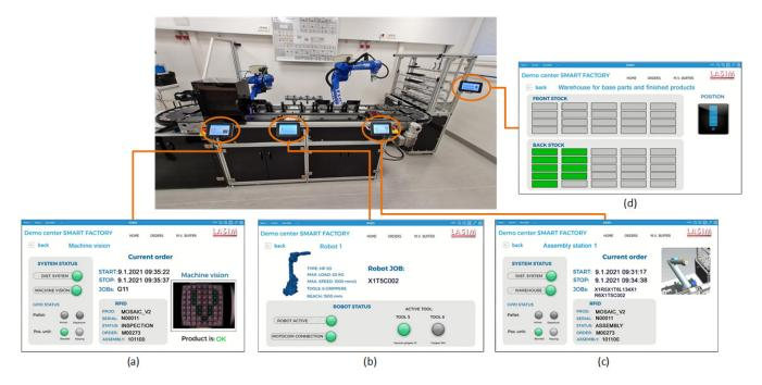
**Figure 18.** Visualization of the processes for the case study for different building blocks in the fourth scenario: (**a**) Machine vision, (**b**) Robot 1, (**c**) Assembly station 1, and (**d**) WBPFP.
