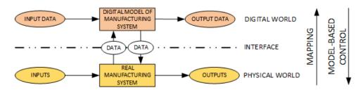
Figure 1. Connections between a real manufacturing system and its digital model.
