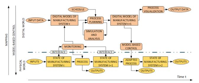
Figure 9. Position of the model and the connections between the physical and digital worlds.
