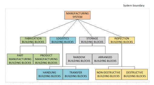
Figure 3. The manufacturing system broken down into four groups of building blocks.
