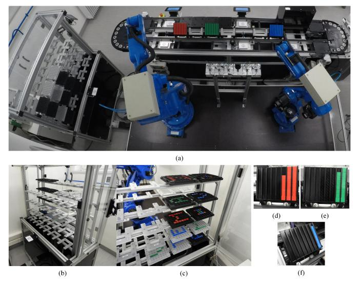
**Figure 16.** The figure shows: (**a**) the state of the assembly system before the start of assembly with full WBPFP and buffers; (**b**) no base parts in the first row of the WBPFP after assembling; (**c**) finished products in the warehouse in the second row; (**d**) the state of the buffer with red tiles, (**e**) green tiles, and (**f**) blue tiles after the completion if the assembly process.
