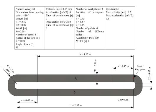
Figure 13. Values used for the digital model of the conveyor.
