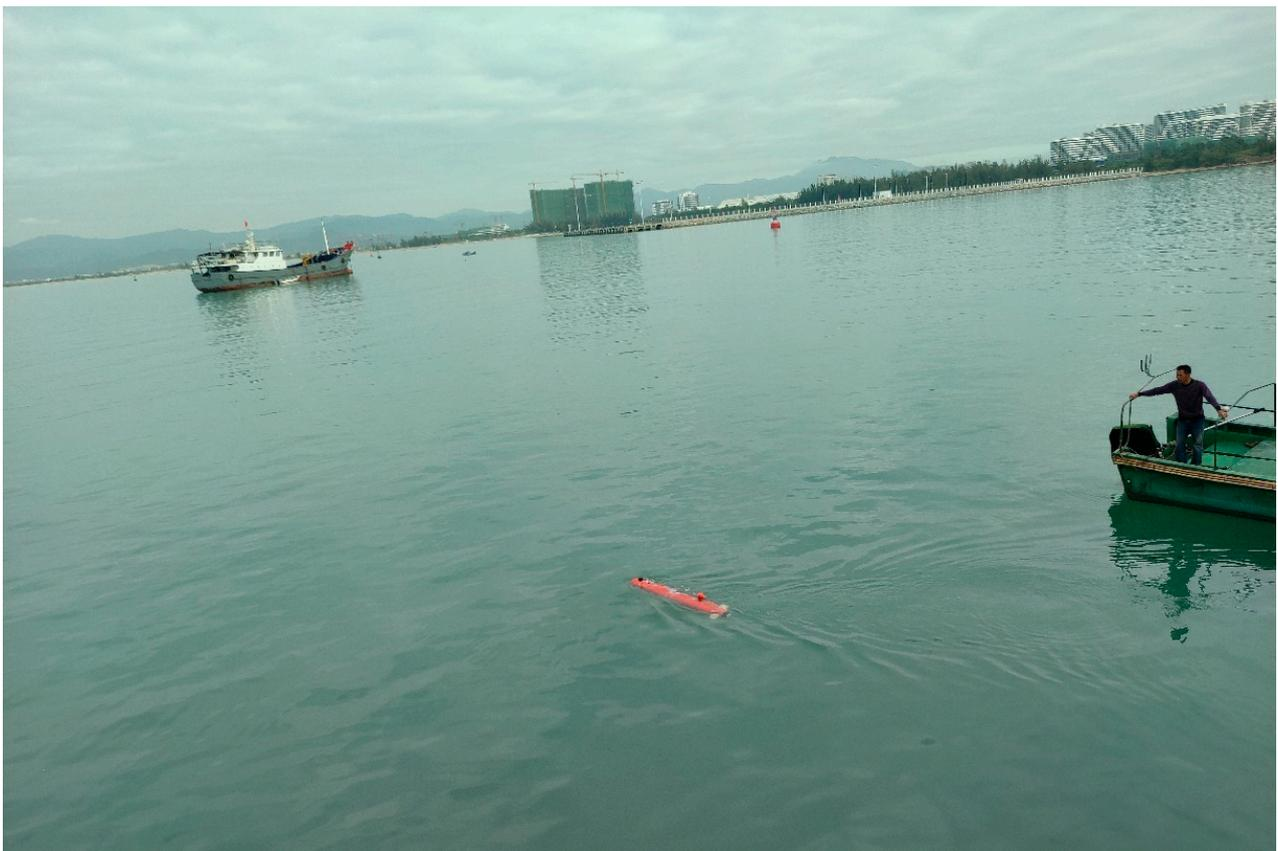
**Figure 16.** The portable AUV in sea trial.
