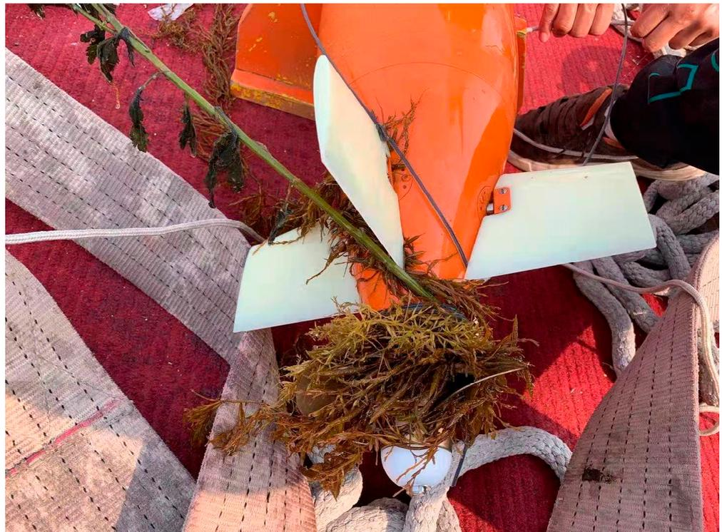
**Figure 18.** Thruster of the portable AUV blocked by weeds during the sea trial.
