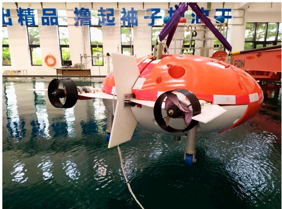
Figure 14. Thruster of the saucer-shape AUV entangled with cloth strips in the pool test.
