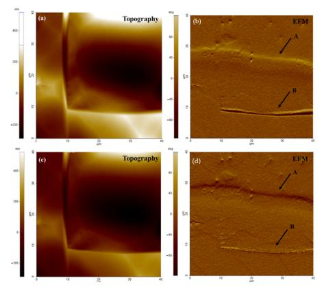
**Figure 5.** Electrostatic force microscopy (EFM) images of  $H_2S$  (600 °C)-treated silicon wafers. (**a**,**b**) were measured under forwarding bias voltage, while (**c**,**d**) were measured under a reverse bias voltage.
