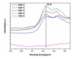
Figure 2. XPS spectra of S 2p for an H<sub>2</sub>S-passivated Si surface.
