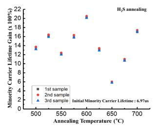
Figure 1. The plot of minority carrier lifetime gains vs. annealing temperature for H<sub>2</sub>S annealing.
