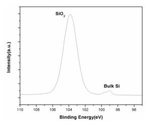
**Figure 3.** XPS spectra of Si 2p for an H<sub>2</sub>S-passivated Si surface (700  $^{\circ}$ C).
