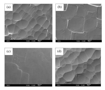
**Figure 4.** SEM images of the silicon surface: (**a**) saw damage etched wafer without  $H_2S$  annealing treatment, (**b**) saw damaged etched wafer under 525 °C  $H_2S$  annealing treatment, (**c**) saw damage etched wafer under 600 °C  $H_2S$  annealing treatment, (**d**) saw damage etched wafer under 700 °C  $H_2S$  annealing treatment.
