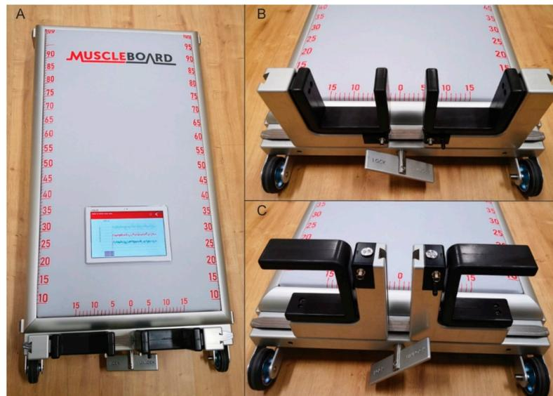
**Figure 1.** Portable dynamometer MuscleBoard®. (A) = the device from above: measurement scales, tablet with software; (B) = sensor braces with load cells in position for measuring horizontal movement (left or right); (C) = sensor braces with load cells in position for measuring vertical movement (up or down).
