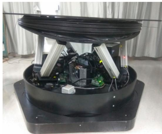
Figure 2. Six degrees of freedom (6-DOF) flight simulation experiment platform.
