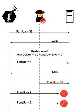
Figure 9. ABP device exploiting the Replay Attack. Adapted from [79].
