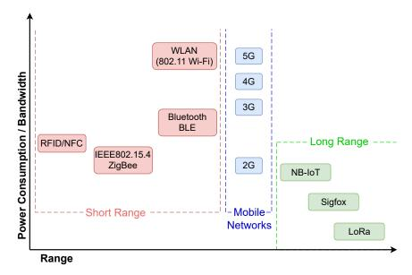
Figure 2. Power/Bandwidth vs. Range in wireless communication Technologies. Adapted from [10].
