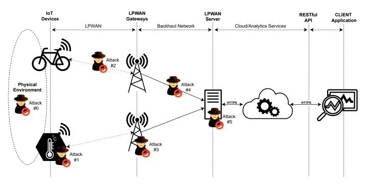
**Figure 12.** Definition of Attack Vectors in Low Power Wide Area Networks (LPWAN)-based Internet of Things (IoT) applications.
