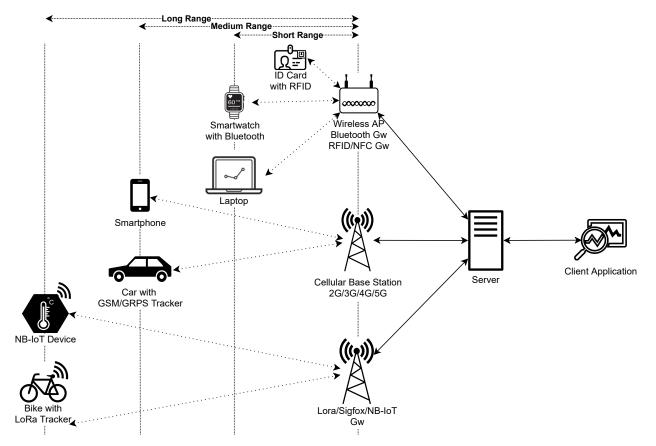
Figure 1. Communication Technologies in IoT applications by range.
