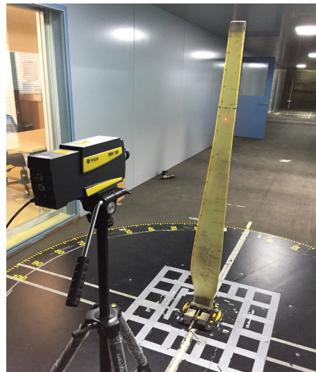
Figure 3. Blade set-up for modal testing based on impact hammer excitation.
