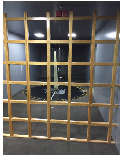
Figure 12. Experimental set-up for wind tunnel experiments: passive grid, blade, and laser vibrometer.
