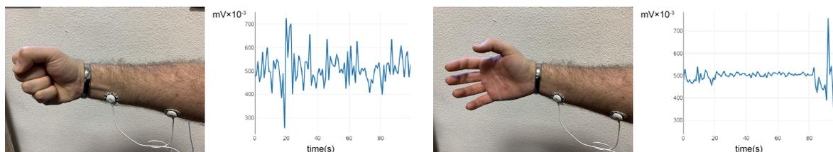
**Figure 2.** Two samples of hand poses and the corresponding sEMG profile, as provided by the BITalino controller. The X-axis shows the time, measured in seconds, and the Y-axis shows the muscle activity, measured in  $\text{mV} \times 10^{-3}$ .
