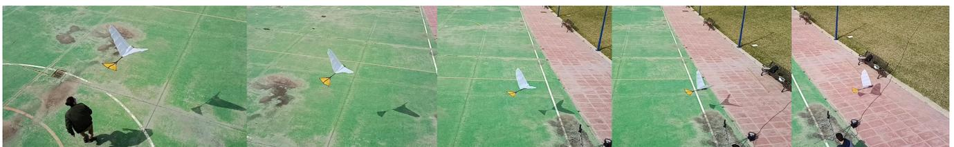
Figure 17. Twist Flapping-Flight Composition Test. Top View.
