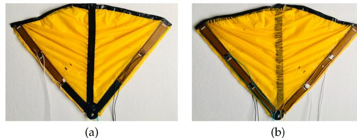
**Figure 5.** Final Developed Tail Model Prototype. (a) Tail upper site. (b) Tail bottom part.
