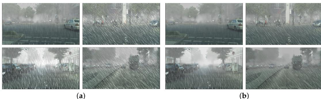
**Figure 3.** Example comparison of synthesis methods on road image using rain-models. (a) Using linear addition model, (b) Using screen blending model.
