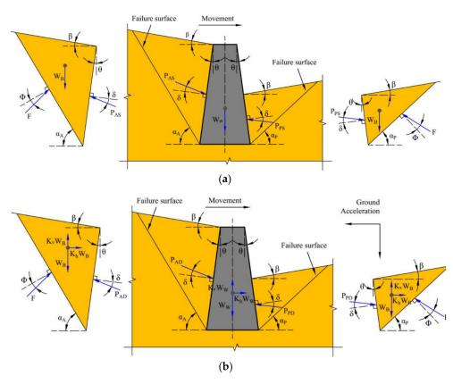
**Figure 1.** Schemes for determining the lateral earth thrust in retaining walls: (a) Coulomb theory [28] (b) Mononobe-Okabe theory [29].
