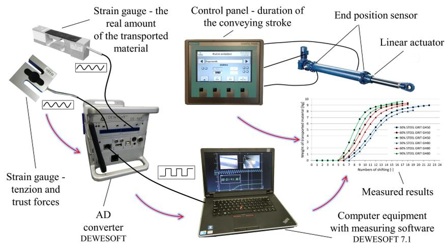
Figure 5. Scheme of the measuring chain with the measuring system, DEWESOFT 7.1.
