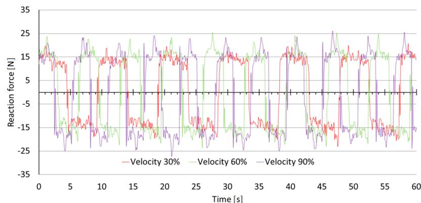
**Figure 6.** Reaction forces acting on the driving mechanism during operation of empty conveyor; the material shifting speeds are adjusted at the levels of 30%, 60% and 90%.
