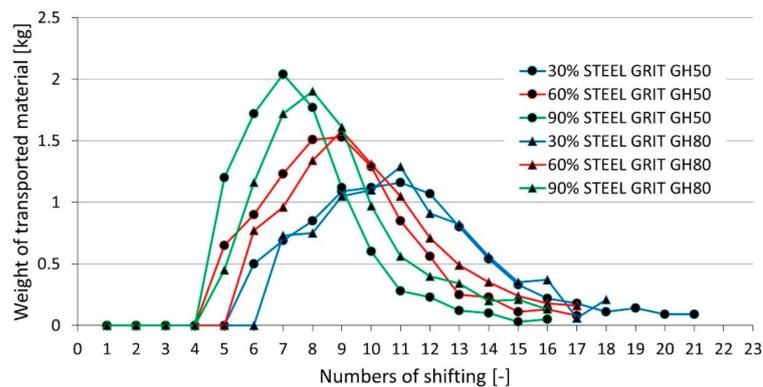
**Figure 12.** Dependence of weight of the transported steel abrasive materials, STEEL GRIT GH50 and GH80, in the case of one stroke on sequence of the stroke during gradual feeding of the conveyor with 10 kg of this material at the 30%, 60% and 90% levels of shifting speed.
