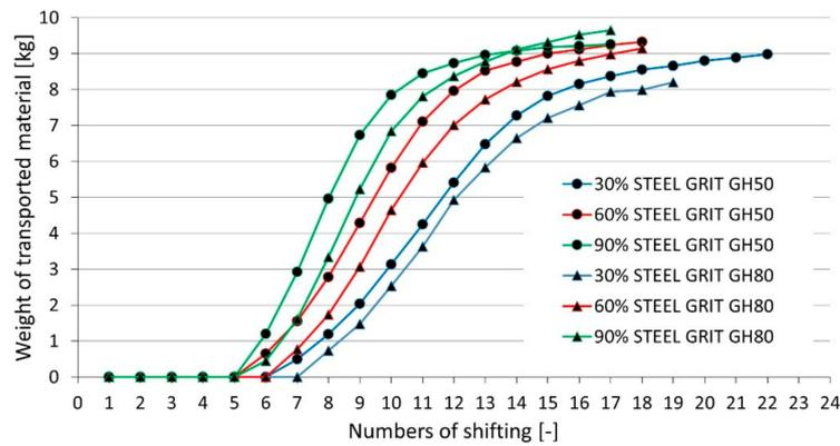
**Figure 9.** Dependence of real weight of the transported materials, STEEL GRIT GH50 and GH80, on number of the strokes during gradual feeding with 10 kg of this material at the 30%, 60% and 90% levels of shifting speed.
