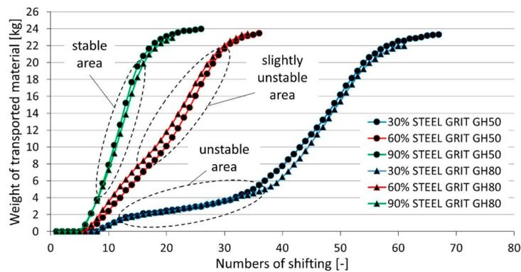
**Figure 10.** Dependence of real weight of the transported materials, STEEL GRIT GH50 and GH80, on number of the strokes during gradual feeding with 25 kg of this material at the 30%, 60% and 90% levels of the shifting speed.
