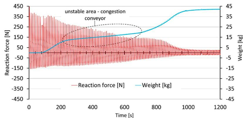
**Figure 8.** Reaction force acting on the driving mechanism at the 30% level of shifting speed for the transported abrasive material, STEEL GRIT GH50, and depending on gradual feeding of the conveyor with 45 kg of the abrasive material.
