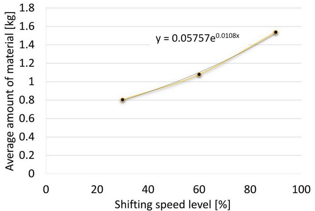
Figure 14. Dependence of the average value for amount of the transported material, STEEL GRIT GH50, in the case of one stroke on the adjusted shifting speed level.
