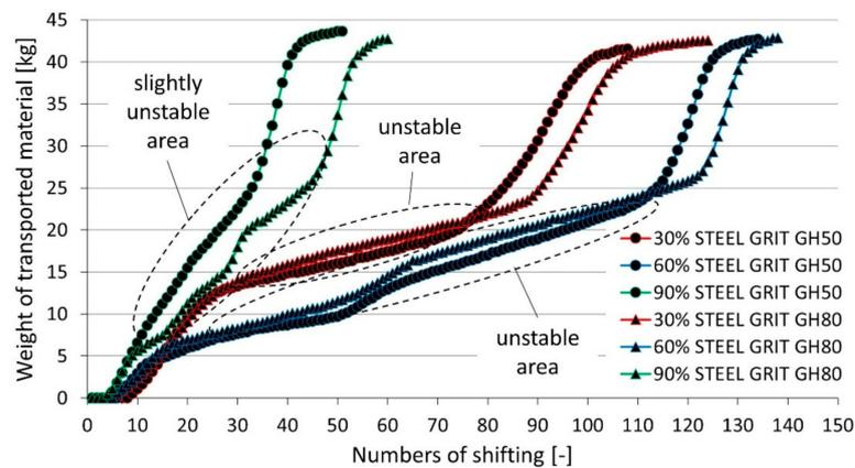
**Figure 11.** Dependence of real weight of the transported materials, STEEL GRIT GH50 and GH80, on number of the strokes during gradual feeding with 45 kg of this material at the 30%, 60% and 90% levels of the shifting speed.
