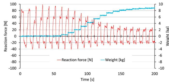
**Figure 7.** Reaction force acting on the driving mechanism at the 30% level of shifting speed for the transported abrasive material, STEEL GRIT GH50, and depending on gradual feeding of the conveyor with 10 kg of the abrasive material.
