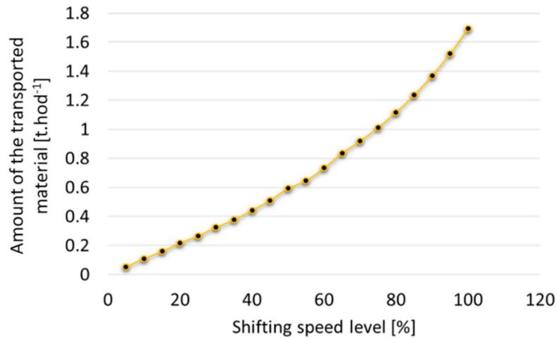
Figure 13. Dependence of the average value for amount of the transported material, STEEL GRIT GH50, on the adjusted shifting speed level.
