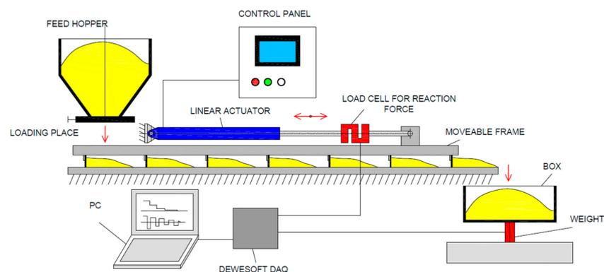
**Figure 3.** Scheme of the experimental testing equipment with the measuring points.
