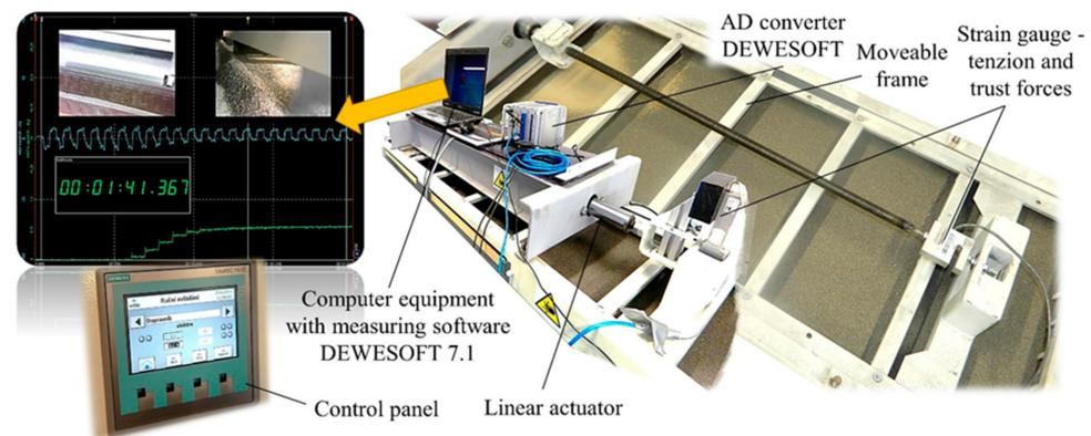
**Figure 2.** Testing equipment with control panel.
