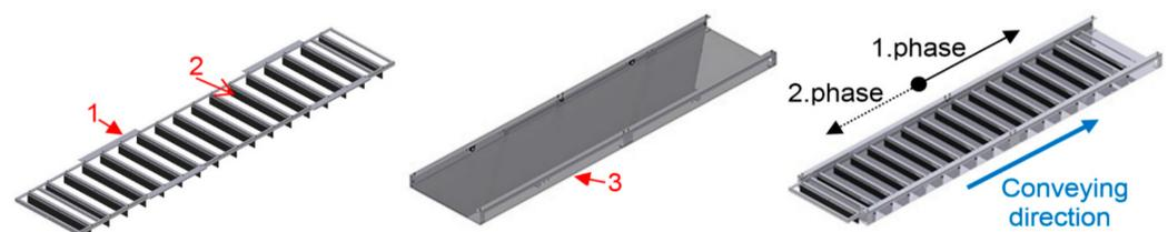
**Figure 1.** Special scraper conveyor without electric drive: 1—moveable frame, 2—scraping membranes and 3—basic static frame.
