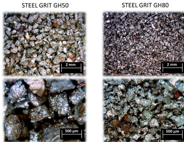
Figure 4. Microscopic photos of the steel abrasive material STEEL GRIT GH50 and Scheme 80.
