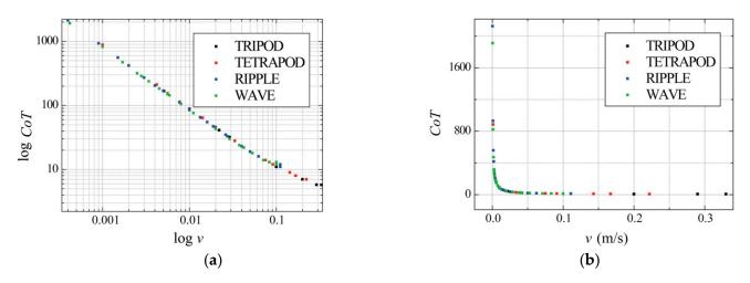
Figure 5. Cost of transport dependence on robot speed: (a) logarithmic scale, (b) linear scale.
