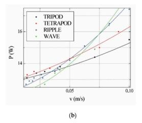
**Figure 3.** Average power dependence on robot speed and gaits: (a) normal view, (b) enlarged view. Experiments were carried out without additional load on the robot. Each dot represents a separate experiment with a certain configuration. Lines show polynomial approximation. No gait type switching was used.
