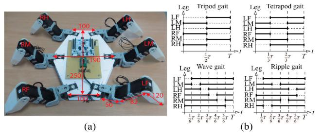
**Figure 1.** Hexapod robot model HexaV4 (a) and gait used in experiments time diagrams (black lines represent leg's support phase, dashed gap—transfer phase) (b). Leg abbreviations: LF—left front; LM—left middle; LH—left hind; RF—right front; RM—right middle; RH—right hind; T—gait period. All dimensions are in millimeters.
