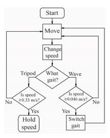
**Figure 2.** Algorithm for switching between wave and tripod gaits. Wave gait is used when the movement speed is lower than 0.046 m/s; tripod gait is used when the movement speed is higher than 0.046 m/s until the speed reaches a maximum value of 0.33 m/s.
