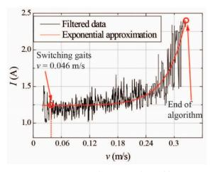
**Figure 6.** Current-time diagram, achieved by varying robot speed and gaits. Black curve—filtered experimental data; red line—exponential approximation.
