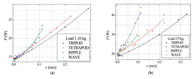
**Figure 4.** Average power dependence on robot speed and gaits with different robot loads: (a) 1.16 kg load, (b) 2.9 kg load. Each dot represents a separate experiment with a certain configuration. Lines show polynomial approximation. No gait switching was used.
