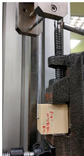
**Figure 3.** Experimental setup. The sawbone was clamped in place and the braided polyethylene lines were tied to a custom-made pulling jig.
