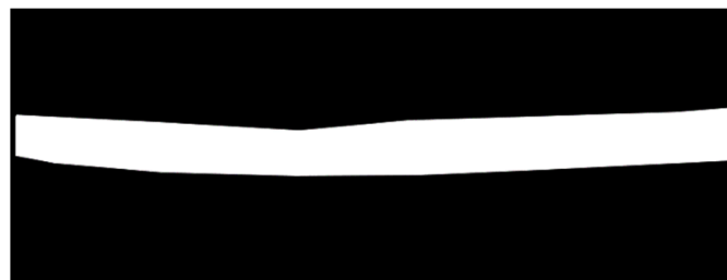
Figure 5. Mask image consisting of pixel intensity 0 of basic metal and 1 of weld bead.
