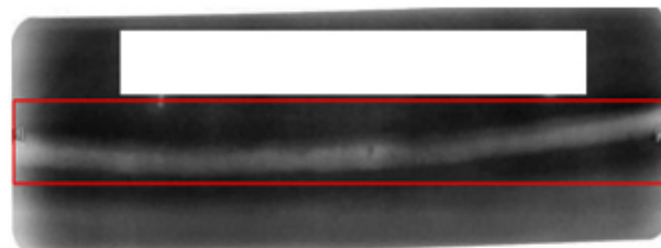
Figure 9. Bounding box image drawn along the bead shape.
