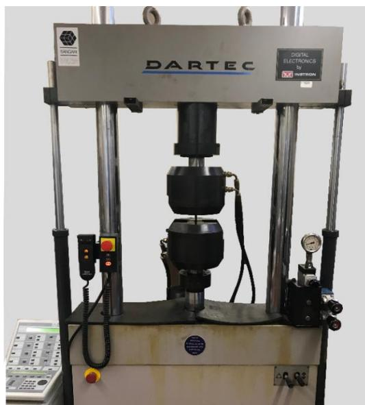
**Figure 2.** Experimental apparatus used in the uniaxial stress-controlled fatigue tests.
