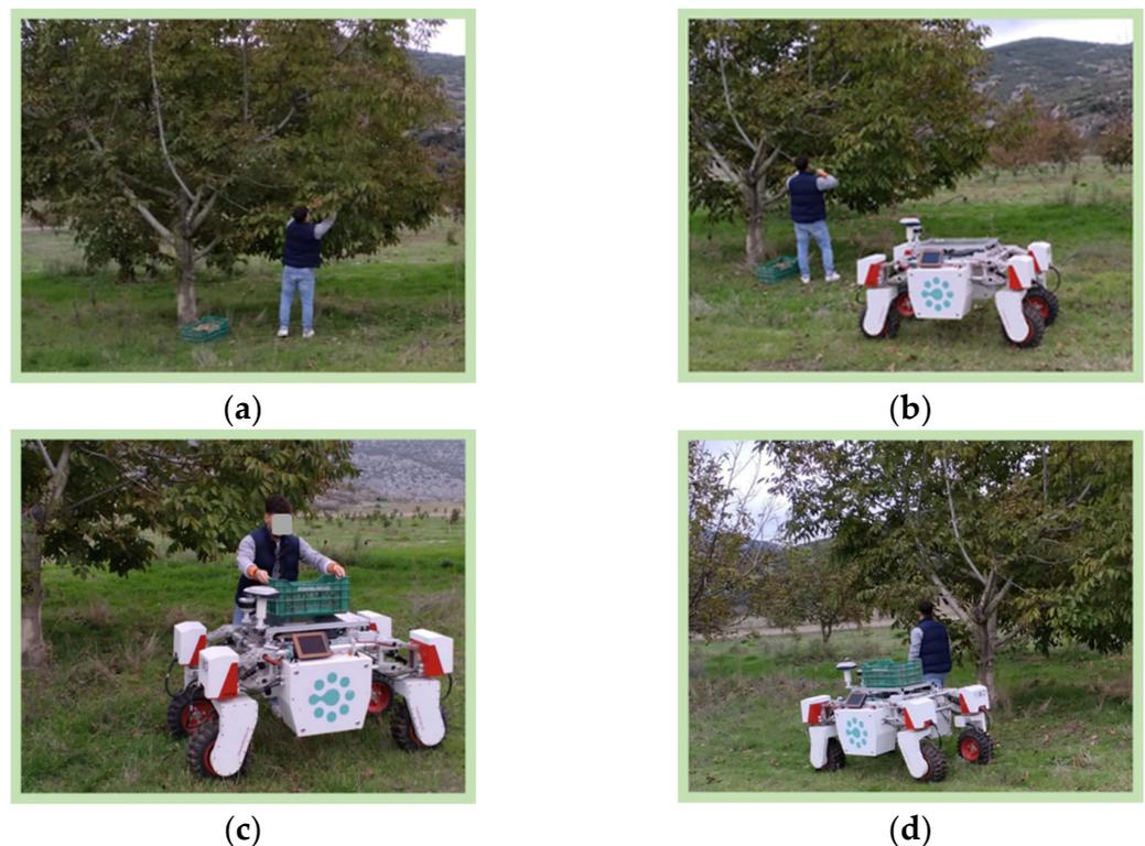
**Figure 1.** Images taken from a pilot study showing: (a) The worker harvesting walnuts, (b) the UGV approaching the worker, (c) the worker lifting the crate onto the UGV, and (d) the UGV carrying the crate towards the desired site.
