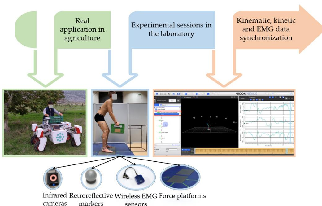
**Figure 2.** Schematic representation of the real application in agriculture and the emulation of the lifting task in a laboratory along with the utilized equipment, and the Vicon Nexus software used for synchronizing the collected data.
