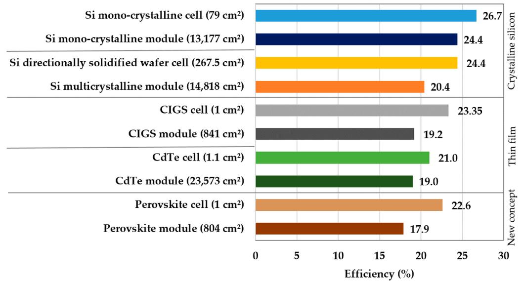
Figure 4. Best cell and module efficiencies found in the literature. Data from Green et al. [69].
