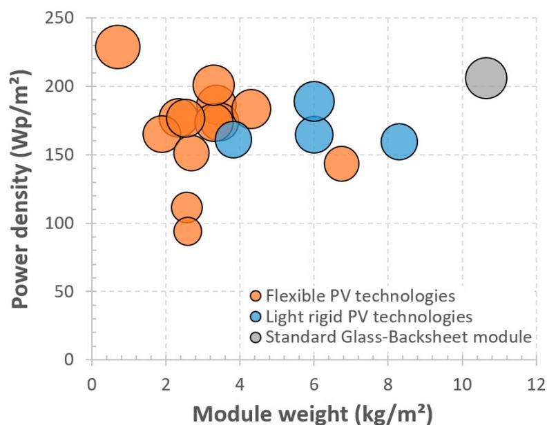
Figure 7. Number of flexible and light (nonflexible) modules in Table 2 (commercial brands) and their weight, where each bubble is a product. The flexible modules do not include the typical 6 kg/m<sup>2</sup> metal sheet of the car body.
