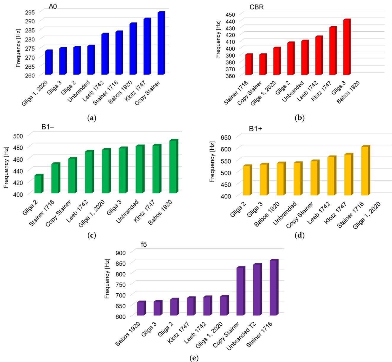
**Figure 9.** Comparisons between the values of the natural frequencies of the tested violins: (a) cavity mode; (b) CBR mode; (c) B1– mode; (d) B1+ mode; (e) the 5th resonance frequency.
