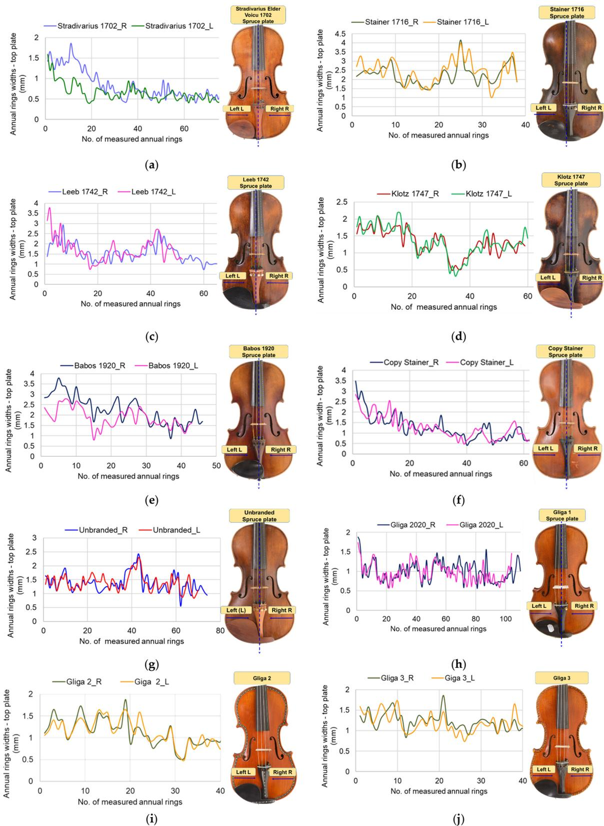
**Figure 6.** Analysis of the symmetry of the anatomical structure of spruce wood in the construction of violin top plate made from resonant spruce: (a) Stradivarius Elder Voicu 1702 violin; (b) Stainer 1716 violin; (c) Leeb 1742 violin; (d) Klotz 1747 violin; (e) Babos 1920 violin; (f) Copy Stainer violin; (g) Unbranded violin; (h) Gliga 1, 2020 violin; (i) Gliga 2 violin; (j) Gliga 3 violin.
