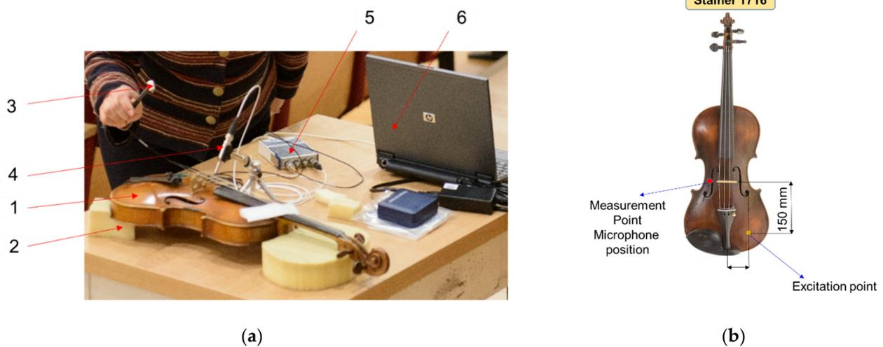
**Figure 4.** Violin testing: (a) excitation with the impact hammer; (b) the positions of excitation and measurement points. Legend: 1—tested violin; 2—elastic support; 3—impact hammer for light structures; 4—microphone; 5—data acquisition board; 6—laptop (software).
