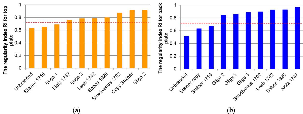
**Figure 7.** Variation of the regularity index: (a) for spruce wood from top plates; (b) for maple wood from back plates of studied violins.
