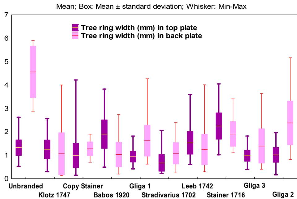
Figure 5. The variation of the annual ring width of the top and back plates of the analyzed violins.
