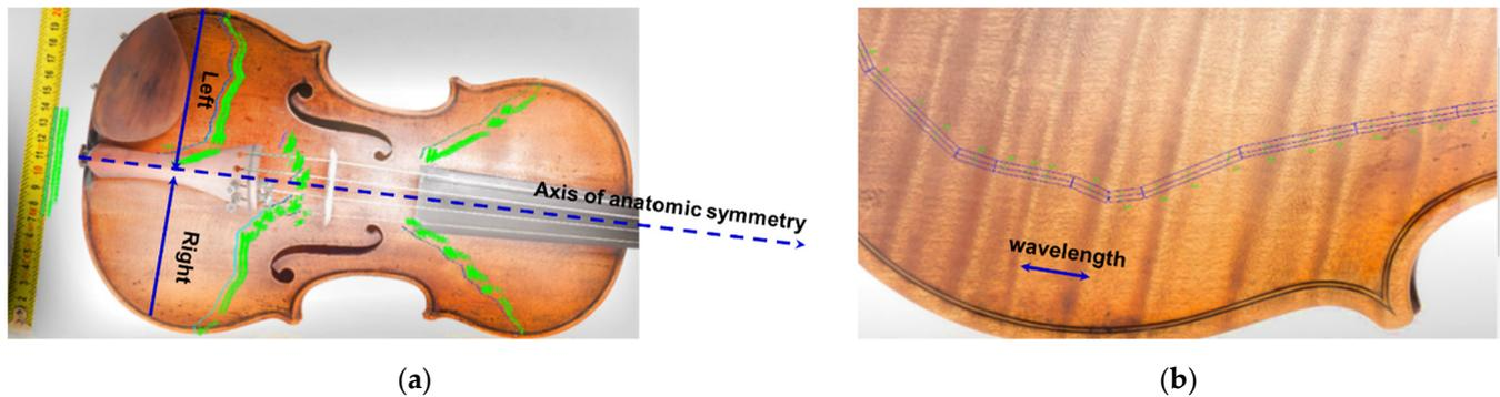
**Figure 3.** How to measure ring rings for the top plates/back plates of violins—case study of the Stradivarius Elder Voicu 1702 (photo courtesy of the “George Enescu” Bucharest Philharmonic and master violinist Tomescu Alexandru): (a) measuring the series of annual rings on the top plate; (b) measuring the wavelength of the curly fiber of maple from the back plate.
