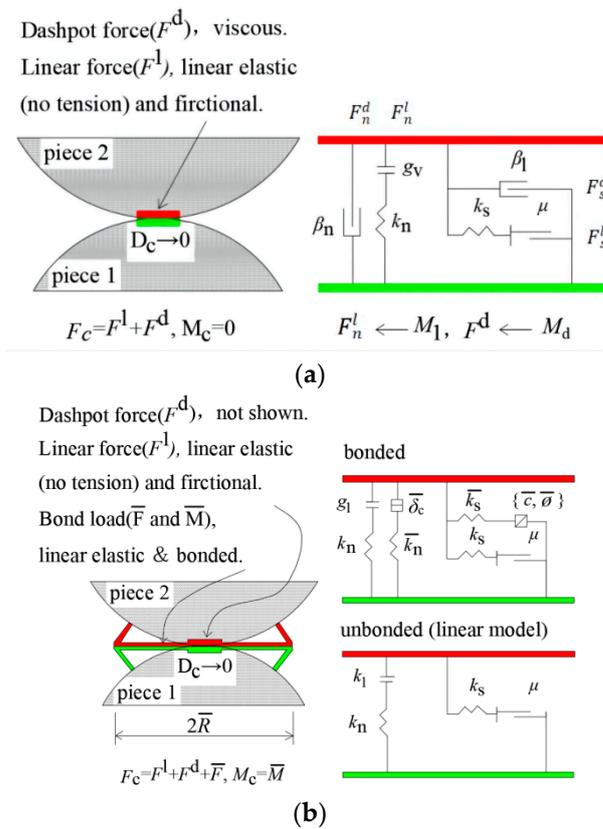
**Figure 6.** Illustration of the model used in this research [27]. (a) the illustration of the linear model; (b) the connection between two different particles is controlled by the linear parallel bond model.
