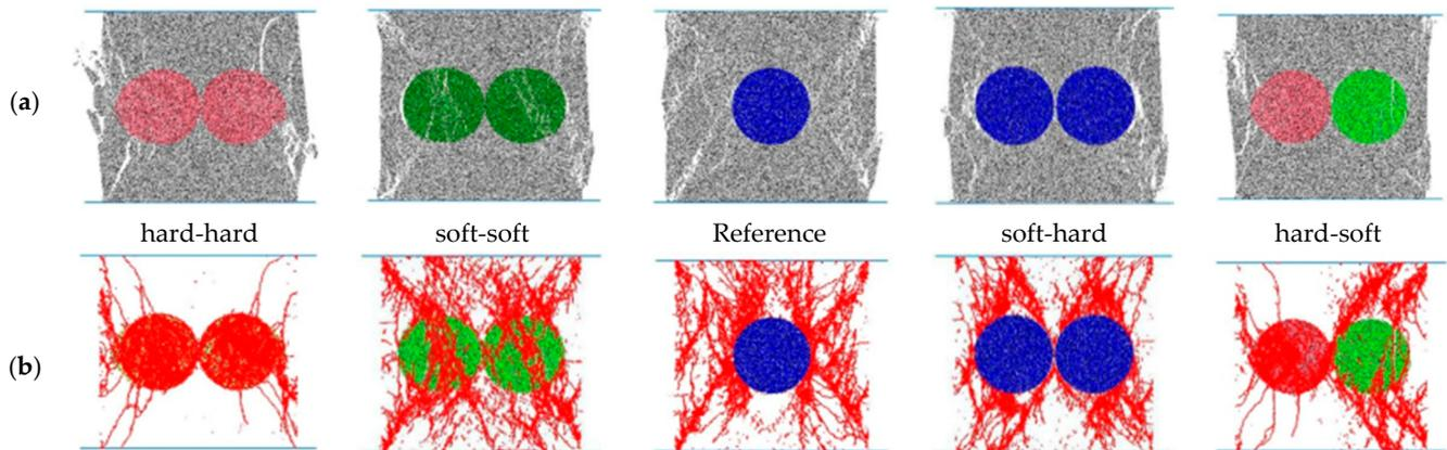
Figure 13. Typical failure modes of specimens in Group 5: (a) failure mode of specimen; (b) failure mode of concretion.
