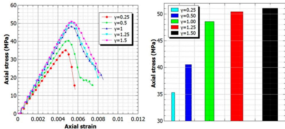
Figure 12. Axial stress, axial strain curves of tested specimens in Group 4.
