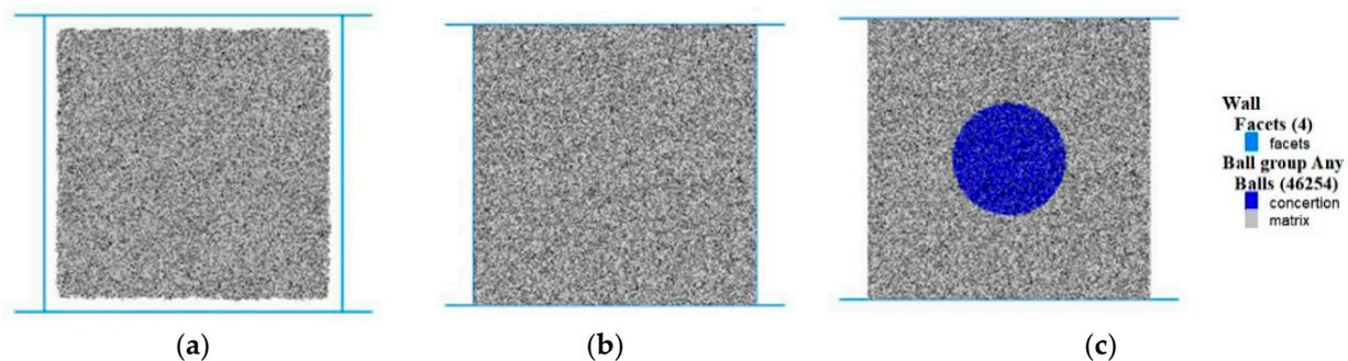
**Figure 4.** Flow chart for the establishment of the specimens: (a) generation of rock mass (matrix); (b) balancing the model; (c) determining and generating the concretion.
