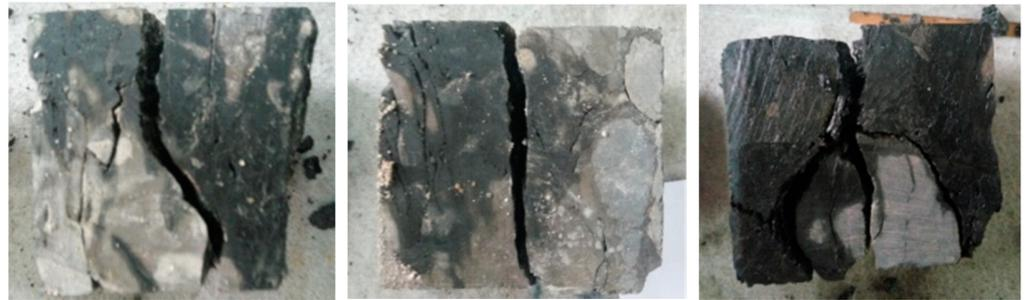
**Figure 2.** Typical failure modes of oil shale specimen ( $50 \times 50 \times 50$  mm) containing the concretions after test.
