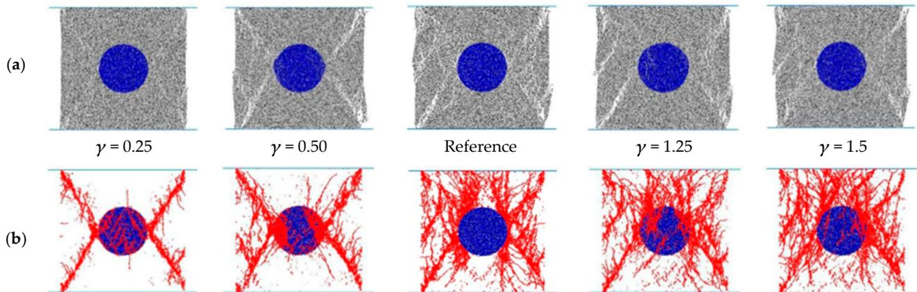
Figure 11. Typical failure modes of specimens in Group 4: (a) failure mode of specimen; (b) failure mode of concretion.
