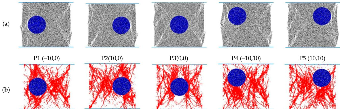
**Figure 9.** Typical failure modes of specimens in Group 3: (a) failure mode of specimen; (b) failure mode of concretion.
