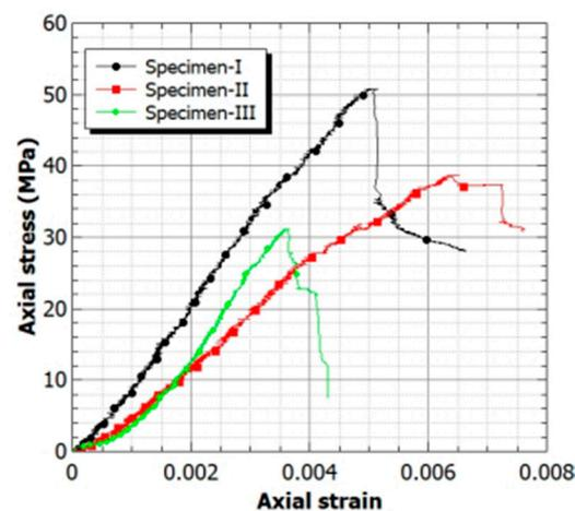
**Figure 3.** Relationship between axial stress and axial strain curves of tested specimens.
