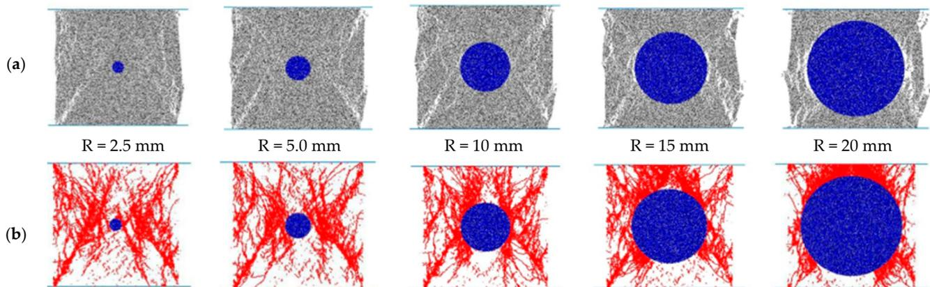
**Figure 7.** Typical failure modes of specimens in Group 2: (a) failure mode of specimen; (b) failure mode of concrete.
