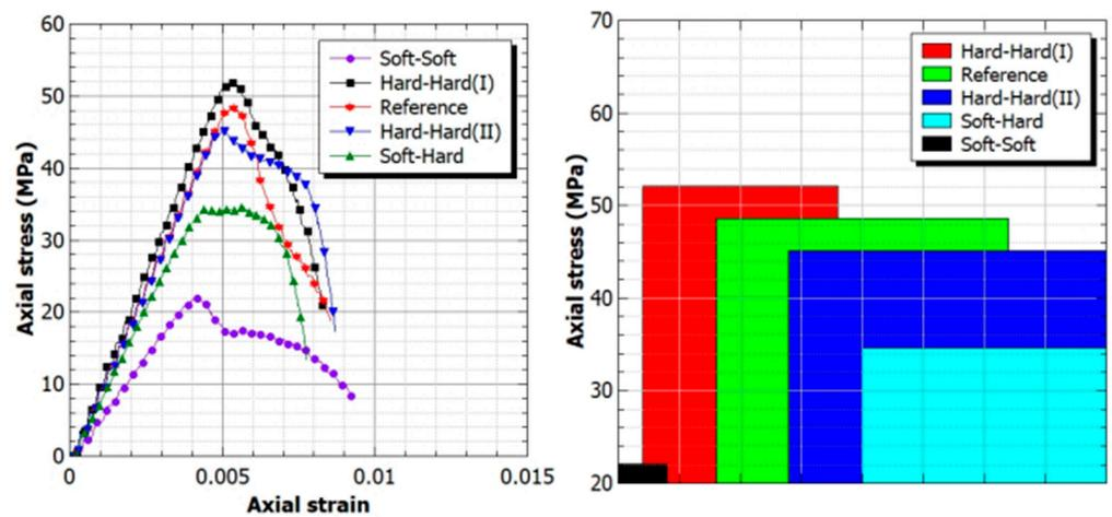
Figure 14. Axial stress, axial strain curves of tested specimens in Group 5.
