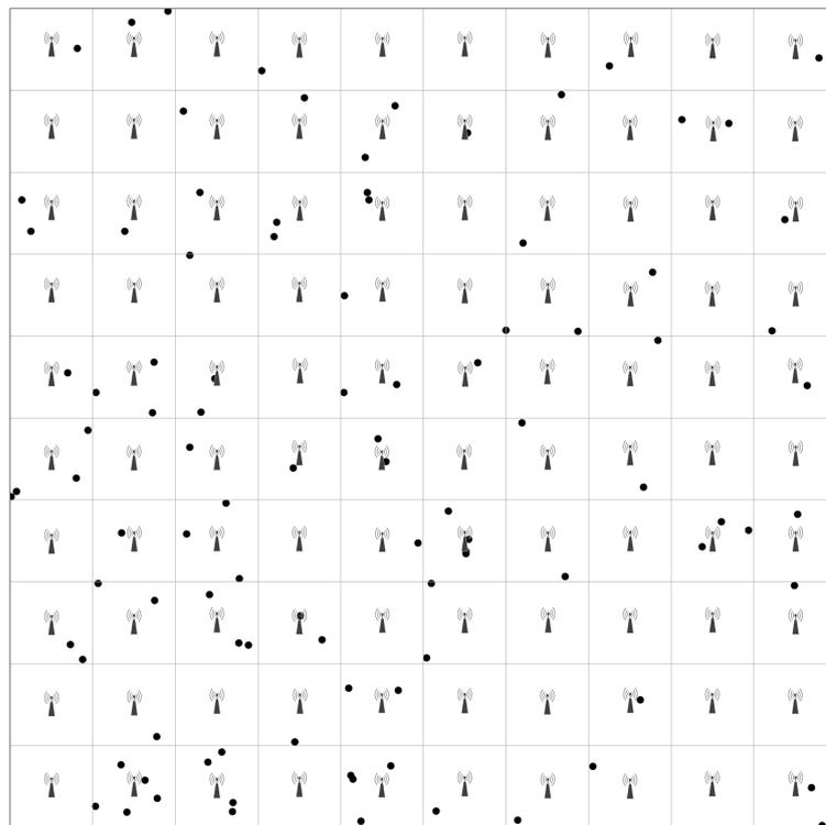
**Figure 7.** The default simulation environment. One-hundred APs are placed in a  $100\text{ m} \times 100\text{ m}$  area, and 100 user stations are randomly deployed inside the area.
