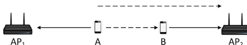
**Figure 3.** An exposed terminal scenario. Node A is exposed to node B, so node B unnecessarily defers its packet even both transmissions can take place in parallel.
