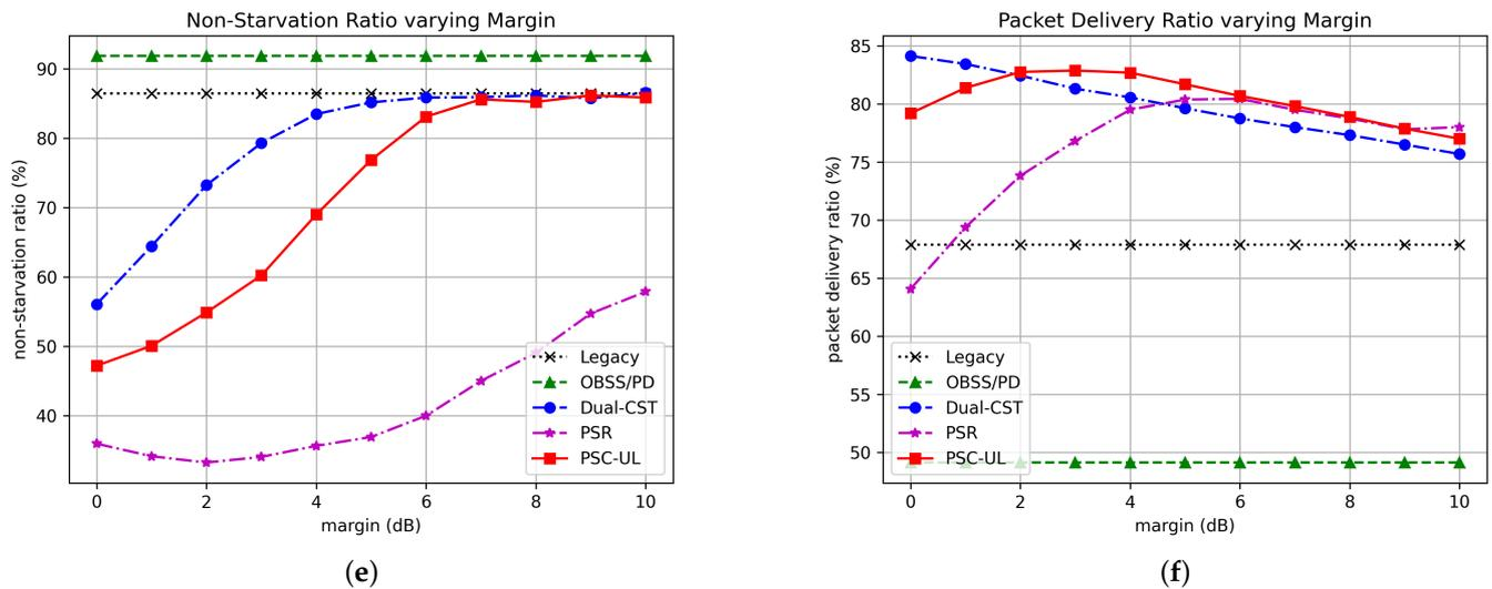
**Figure 12.** Performance of methods varying margin. (a) Total throughput; (b) Bottom 50% throughput; (c) Bottom 25% throughput; (d) Fairness; (e) Non-starvation Ratio; (f) Delivery Ratio.
