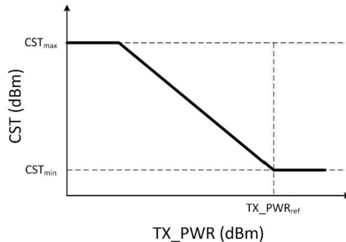
**Figure 1.** CST selection with transmit power control in the OBSS/PD method.
