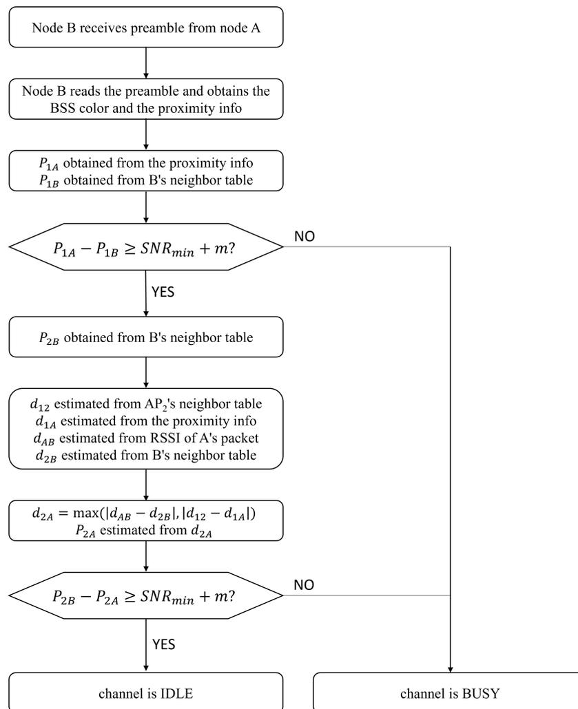
**Figure 6.** A flow diagram illustrating the operation of the proposed method.
