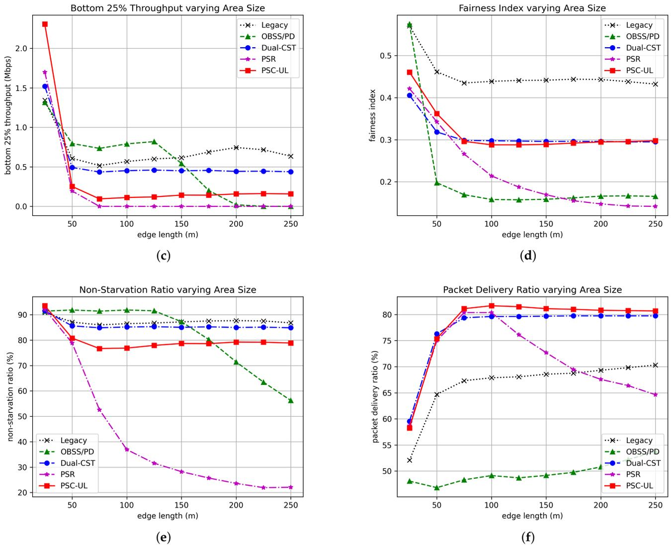
**Figure 11.** Performance of methods varying area size. (a) Total throughput; (b) Bottom 50% throughput; (c) Bottom 25% throughput; (d) Fairness; (e) Non-starvation Ratio; (f) Delivery Ratio.
