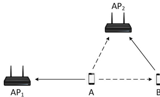
**Figure 4.** A scenario where node B transmits in parallel with node A according to PSR, but node B's packet is lost due to low SNR at AP<sub>2</sub>.
