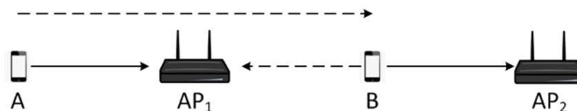
**Figure 2.** A hidden terminal scenario. Node B is hidden to node A, and the packet at AP<sub>1</sub> is lost when both node A and B transmit together.
