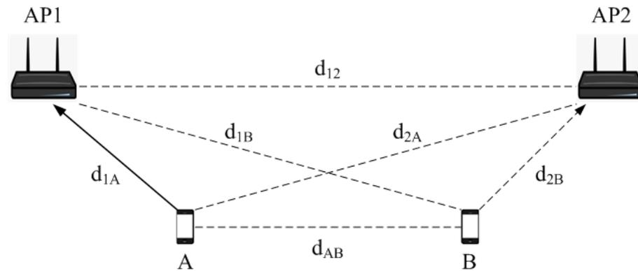
**Figure 5.** A scenario illustrating how a node determines concurrent transmission in the proposed method.
