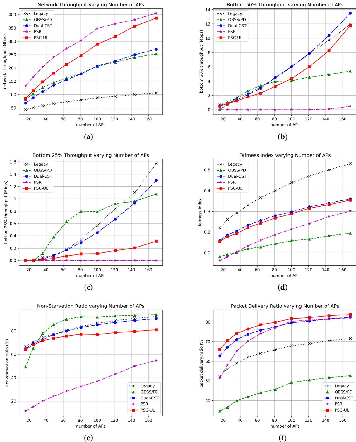
**Figure 10.** Performance of methods varying number of APs. (a) Total throughput; (b) Bottom 50% throughput; (c) Bottom 25% throughput; (d) Fairness; (e) Non-starvation Ratio; (f) Delivery Ratio.
