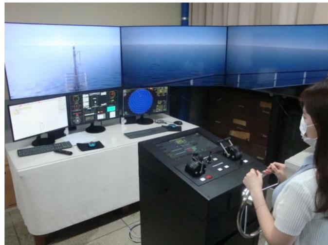
**Figure 4.** Scene of ship maneuvering simulation for observing the turning circle.
