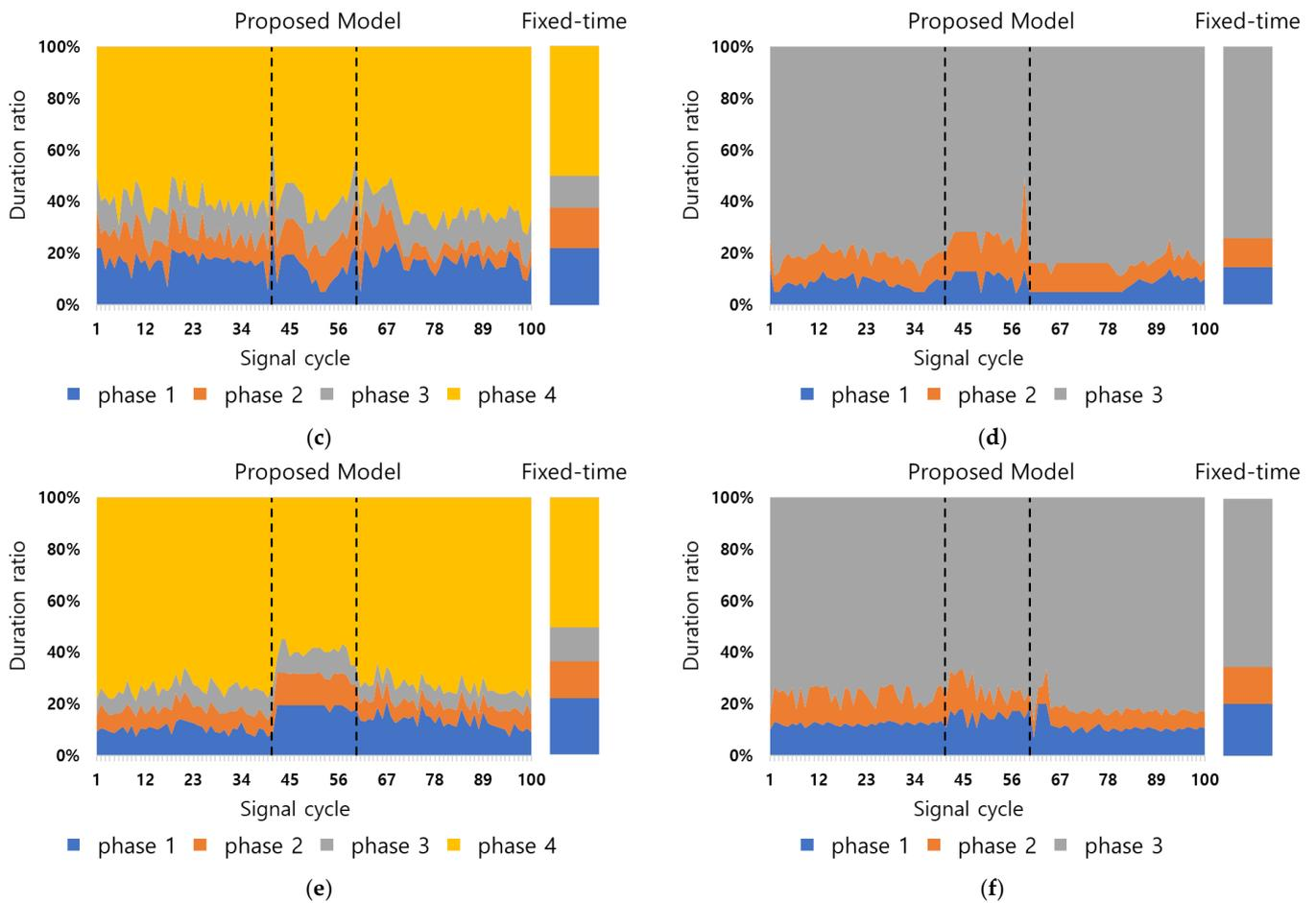
**Figure 6.** Phase duration ratio of scenario 2: (a) Intersection 1; (b) Intersection 2; (c) Intersection 3; (d) Intersection 4; (e) Intersection 5; and (f) Intersection 6. The time point at which the cycle length changes is indicated by a dotted line. The first cycle length is 160 s and changes to 180 s after the first dotted line, and then changes back to 160 s after the second dotted line.
