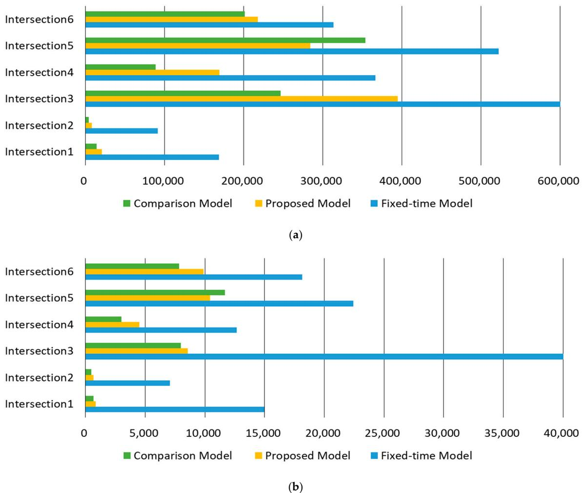
Figure 7. Measure of effectiveness by intersections: (a) Cumulative delay; (b) Cumulative number of stops.
