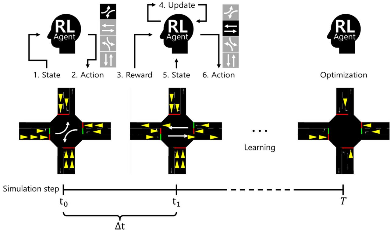
Figure 1. Learning process of the reinforcement learning-based traffic signal control model.
