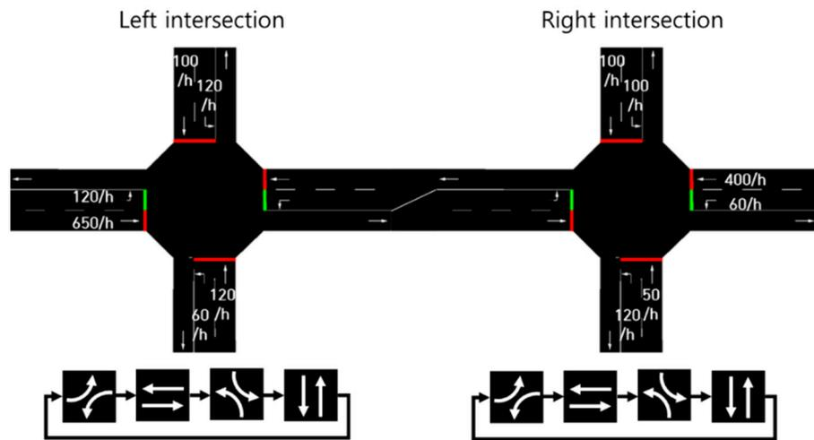
Figure 3. Simple network with two intersections.
