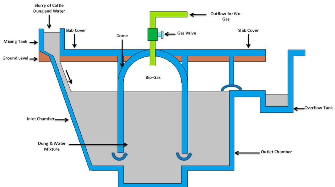
**Figure 6.** Fixed dome types of biogas plants in India.
