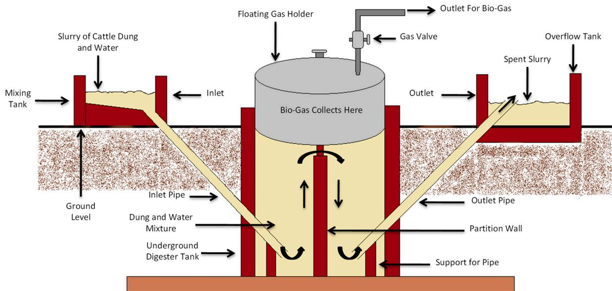
Figure 5. Floating dome types of biogas plants in India.
