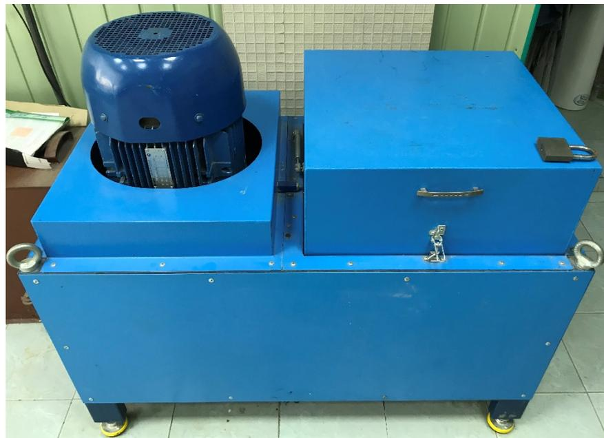
Figure 2. General view of the planetary ball mill “Activator—4M”.
