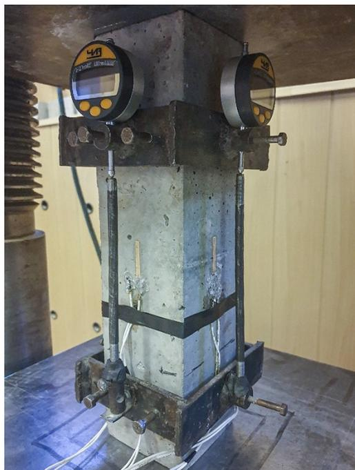
**Figure 4.** The process of measuring concrete deformations.
